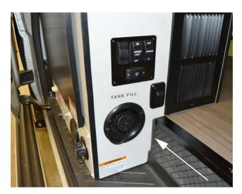
Water Tank Gravity Fill (Located near sliding entrance door)
