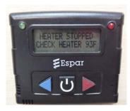
Hydronic Heating System Diagnostic Tool (Located below dinette seat - remove screws and panel to access)
