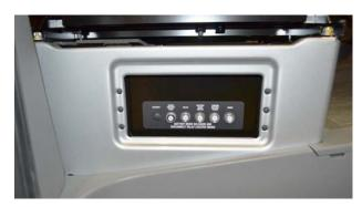
Automotive Chassis 12-Volt Circuit Breakers (Located on outboard side of passenger seat)
