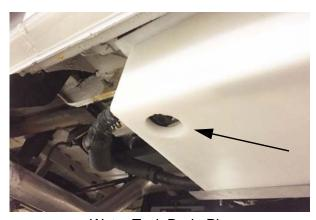
Water Tank Drain Plug (Located beneath running board, behind front passenger side door) -Typical installation shown
