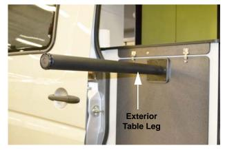
While holding the exterior table leg, release both storage latches and lower table to the ground.
