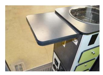
4. Disengage security lock (located beneath countertop extension).
