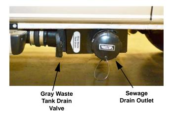
Holding Tank Drain Valves (Located on driver side behind rear tire)
