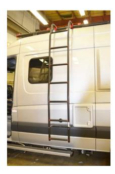
Shown with Ladder properly mounted on rail at driver side rear
