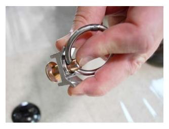
2. Slide tie-down ring into the floor bracket, then release the top of the tie down ring to secure into the floor bracket.
