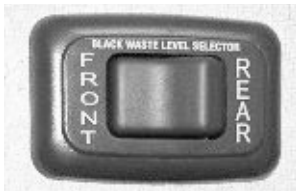
Black Waste Level Selector Switch (Located near monitor panel)
