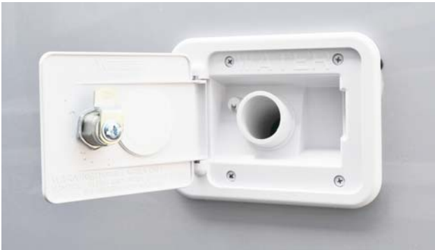
Water Tank Gravity Fill -Typical View
