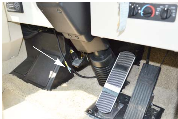
CB Power Wires -Typical View
