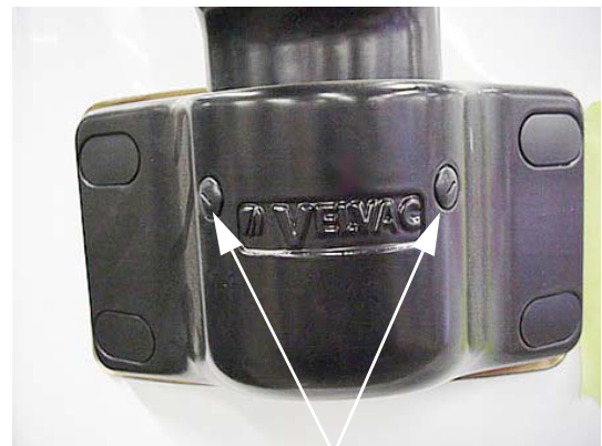
Unscrew protective caps and loosen Allen head set screws to pivot mirror arm. (Torque screws to 75-100 in./lbs.)
