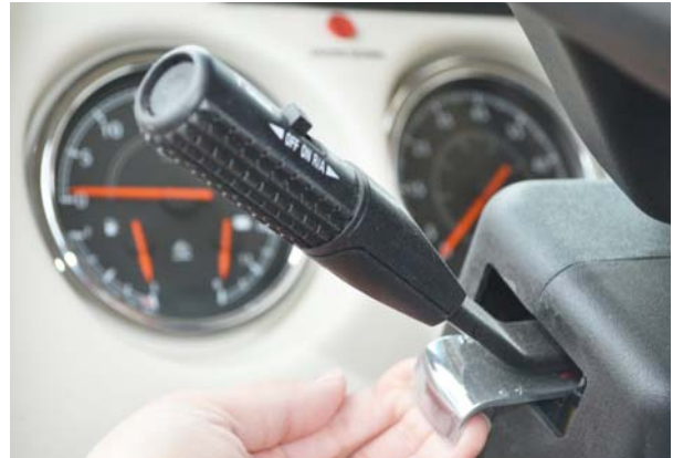
Hazard Warning Flashers (Typical View - your coach may differ depending on model)
