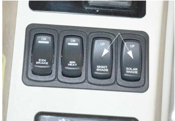
12-Volt Front Drop-Down Solar/Night Shade Switches (Located on driver side trim panel) -Typical View
