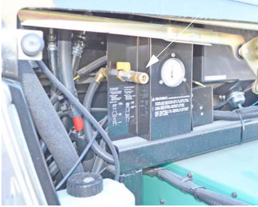
Quick-Connect Air Coupler (Located behind front hood panel) -Typical installation shown
