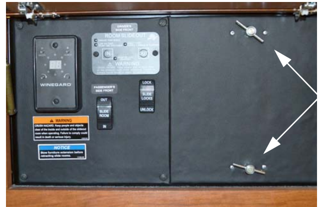
Access Panel Cover Latches Turn “counter-clockwise” to remove cover.
