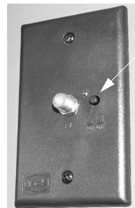
TV Signal Amplifier Power Switch (Located in overhead cabinet above entrance door) -Typical View
