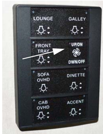
Power Roof Ventilator Switch
