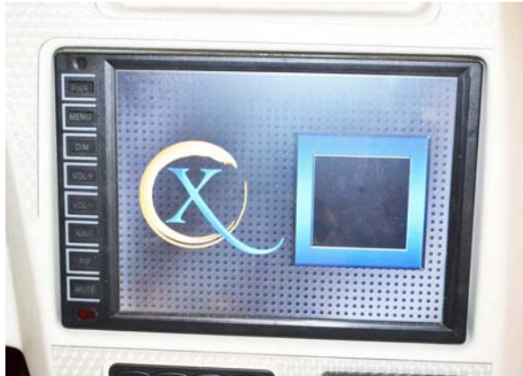
Radio/Rearview Monitor (Located on dash) -Typical View
