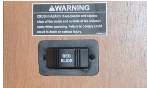
Bed Slide Control Switch (Located on forward bedroom wall) -Typical View
