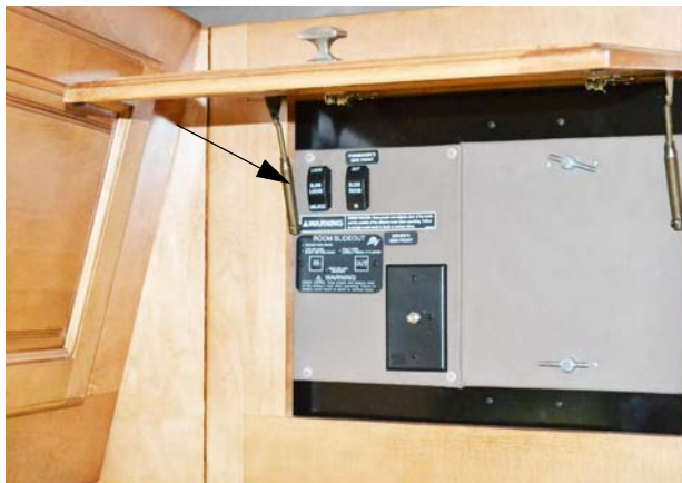
Slideout Room Travel Locks (Your model may be equipped with one or more types) -Typical View
