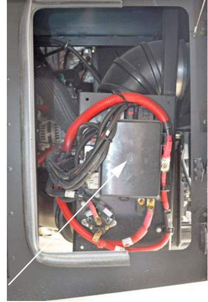
Towing Package Fuses (Located in driver side rear compartment) -Typical View
