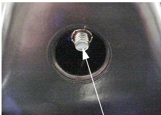
Mirror Arm Pivot Bolt on underside of mounting base - Shown with access plug removed (Torque nut to 75-100 in./lbs.)
