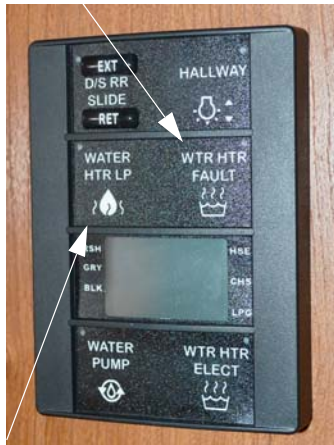
Gas Water Heater Switch (Located on Systems Monitor Panel) -Typical View
