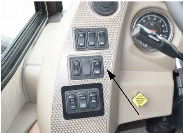
Front AUX Switch (Located on dash) -Typical View
