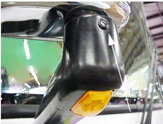
Unscrew protective cap and loosen Allen head set screw to pivot mirror head
