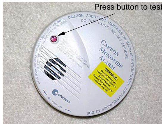
Carbon Monoxide Alarm
