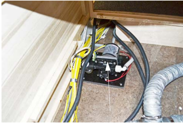
Water Pump (Located beneath removable access panel below bed) -Model 23L shown
