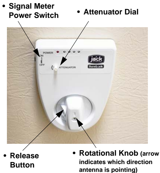
Digital Antenna Signal Meter (Located on ceiling)
