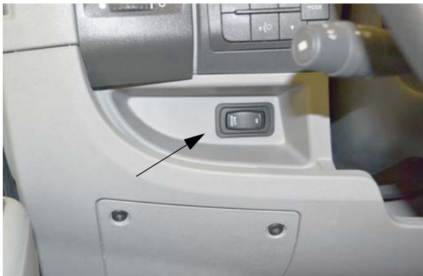
Battery Boost Switch (Located on dash)
