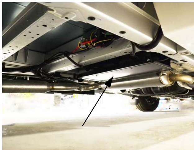
House Battery Access (Located under center of coach) - Remove bolts from battery retainer to remove house battery -Typical View
