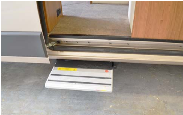
Entry Step (Located near sliding door) -Typical View (Extended position shown)
