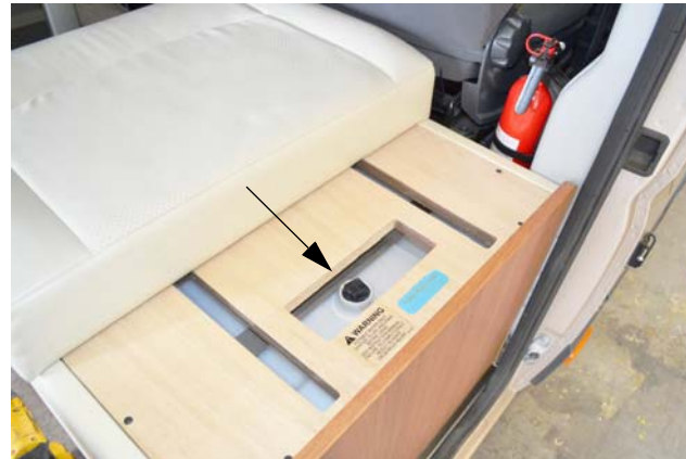
Water Tank Gravity Fill (Located beneath sliding cushion on right dinette seat) -Typical View
