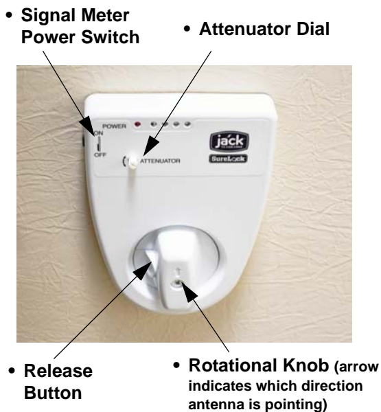
Digital Antenna Signal Meter (Located on ceiling)
