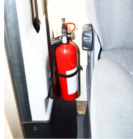
Fire Extinguisher (Located near sliding entrance door) -Typical installation shown
