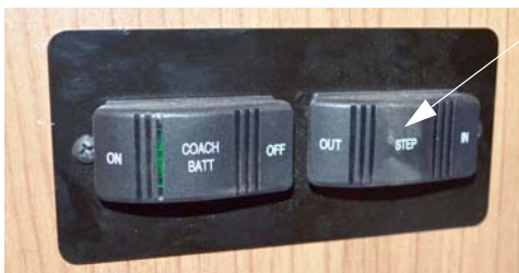
Entry Step Switch (Located near sliding door) -Typical View
