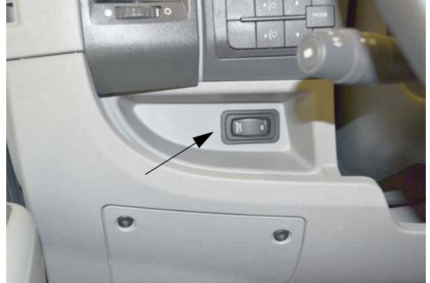
Battery Boost Switch (Located on lower dash area)
