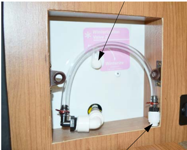
Antifreeze Siphon Tube/Winterization Port (Located front of galley behind access door)
