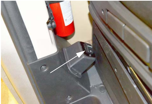
Second Power Awning Switch (Located near right side of passenger seat) -Typical View
