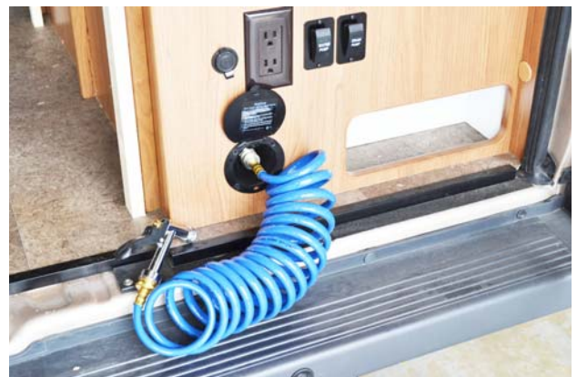
Exterior Shower/Wash Station (Typical)
