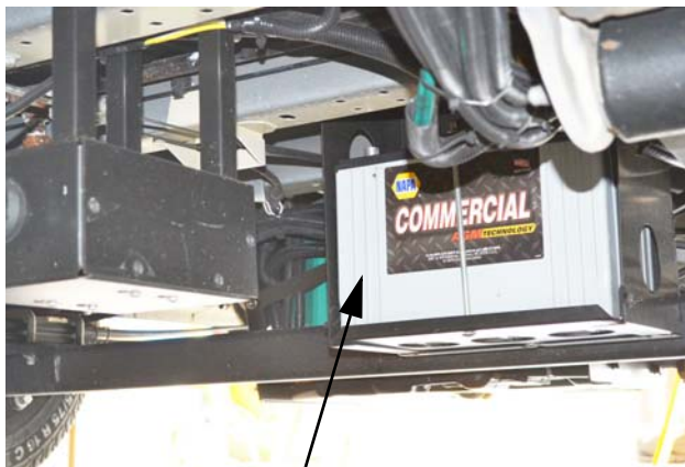
House Battery Access (Located behind rear driver side tires) - Remove bolts from battery retainer to remove house battery
