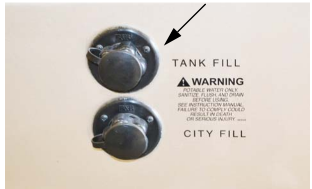
Tank Fill Inlet (Located on the left sidewall)
