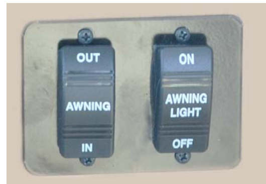
Power Awning and Awning Light Switch (Located at front of galley or shower wall) -Typical View
