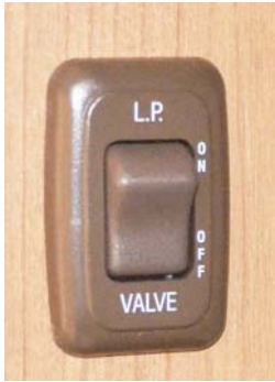
LP Tank Valve Switch
