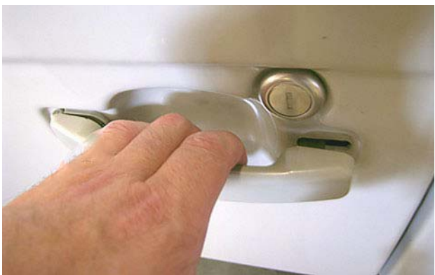
Pull door handles out to unlatch door
