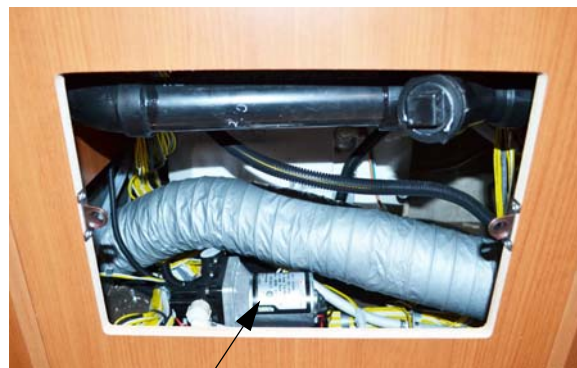
Water Pump (Located behind removable access panel below wardrobe) -Model 24J shown
