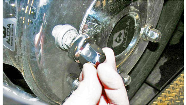
Remove the push on nut covers.
