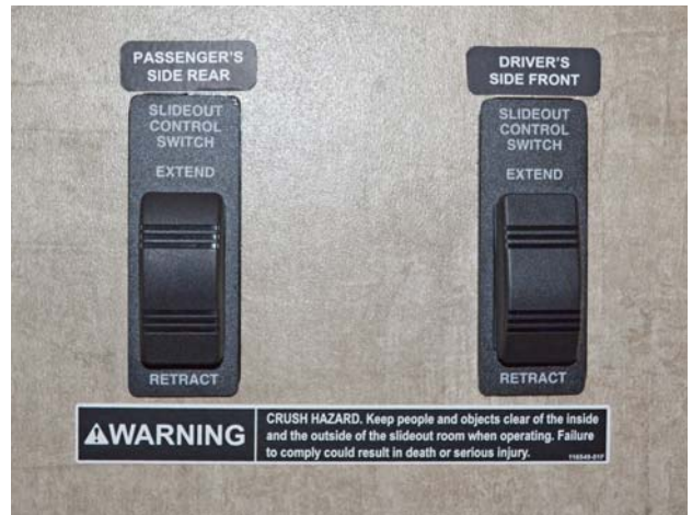
Slideout Switch (Your coach may have one or more slideout switches depending on model, options, and available equipment) -Typical View
