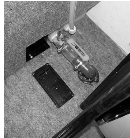
Water Tank Drain Valve (Located in first passenger side compartment) -Typical installation shown
