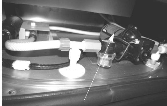
Water Pump (Located in driver side front compartment) -Typical installation shown
