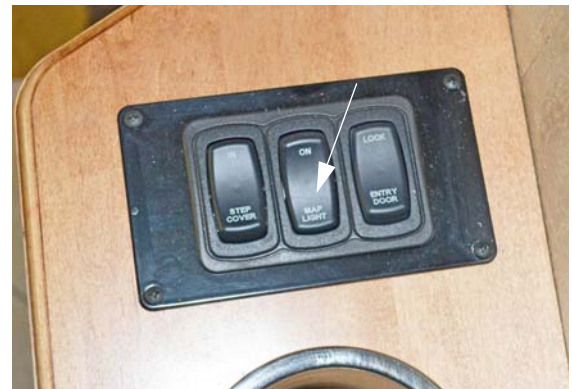
Passenger Map Light Switch (Located on passenger side trim panel) -Typical View
