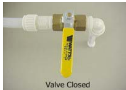
Water Tank Drain Valve (Located in first passenger side compartment) -Typical installation shown
