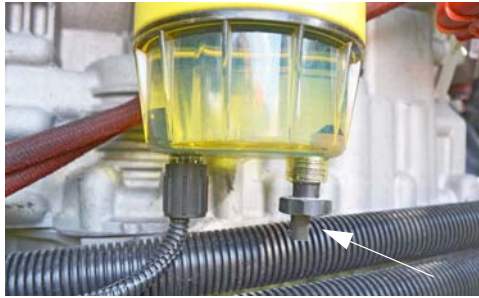
Fuel/Water Separator Drain Valve (Located on bottom end of separator)
