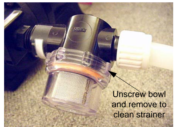
Water Pump Strainer -Typical View
