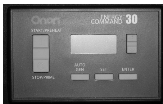
AGS Control Pad (Located near monitor panel)
