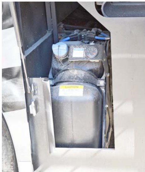
Diesel Exhaust Fluid Fill Tank (Located in passenger or driver side compartment behind rear wheel, depending on model)
