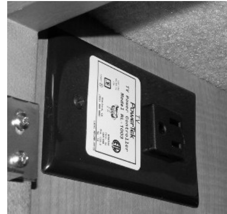
Front TV Ignition Switch Interlock -Typical View
