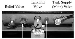
Tank Gauge Overflow and Sender Valve Propane Tank Features (Typical)
