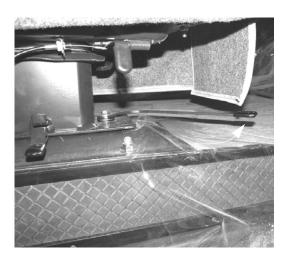
• Tip the seat rearward until the lock pin clears the floor plate locking ramp, then re-lock the Locking Arm to avoid bending.
