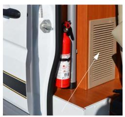
Water Pump (Located behind removable vent on front side of shower cabinet) \* Model 70X
