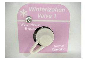
Leave bypass valve handle in NORMAL FLOW position if draining water and blowing out waterlines. Place in BYPASS position ONLY when using antifreeze solution in waterlines.
