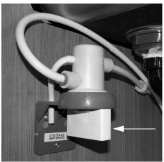
Diverter Plug (installed in filter socket) • Insert and twist 1/4 turn "clockwise".
