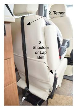
3. Route the shoulder or lap belt through the child seat. Fasten the shoulder or lap belt and pull snug. The locking tab automatically holds the belt in place.
