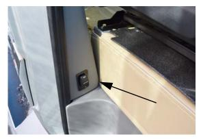
Second Power Awning Switch (Located near right side of passenger seat) -Typical View
