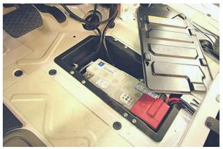
Chassis Battery Access (Located in compartment "well" ahead of driver seat)
