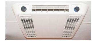
Your coach may be equipped with an air source heat strip built into the air conditioning system. Because the heat strip operates on electricity, it provides economical heat inside your coach and helps reduce the use of propane gas for heating in cooler weather.
