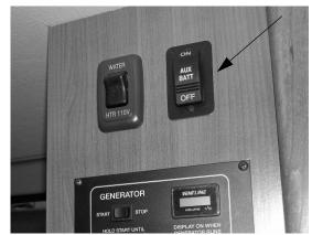
House/Coach Battery Disconnect Switch (Located near monitor panel)
