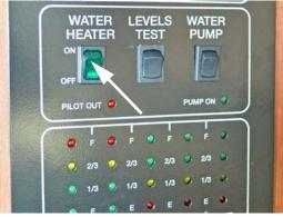
Gas Water Heater Switch (Located on Systems Monitor Panel)
