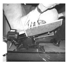
• With the seat tilted slightly rearward, remove the seat assembly by lifting it up and forward.
