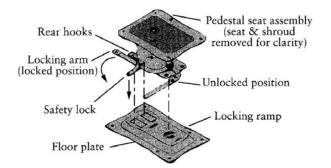
• Press DOWN on the Safety Lock and support seat while rotating the Locking Arm COUNTER-CLOCKWISE, until the arm contacts the stop pin (unlocked position).
