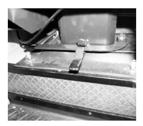
NOTE: Anytime that the Companion Seat is in the vehicle, it must be in position with the Locking Arm in the LOCKED position, and captured by the Safety Lock.
