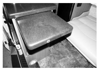
3. Disengage security lock (located beneath countertop extension).
