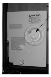
Water Tank Gravity Fill (Located near sliding entrance door) -Typical View
