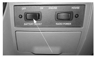
Battery Boost Switch (Located on lower dash area) • Press and Hold in the ON position while turning ignition key for emergency starting power.
