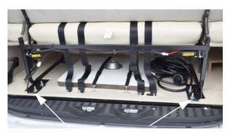
Tether Anchor Loop (Located on each end of sofa) - Open rear doors to access
