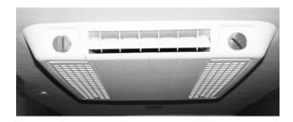
Your coach may be equipped with an air source heat pump built into the air conditioning system. Because the heat pump operates on electricity, it provides economical heat inside your coach and helps reduce the use of propane gas for heating in cooler weather.
