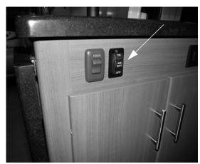
House/Coach Battery Disconnect Switch (Located on front side of galley)
