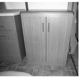
Removable Wardrobe Cabinet (Installed in place of inboard Companion Seat)
