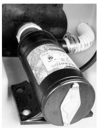
Waste Pump (Located beneath coach) -Typical View
