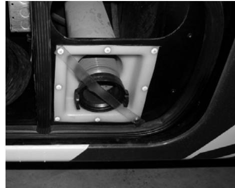
Sewage Drain Hose (Located in front driver side compartment) -Typical View
