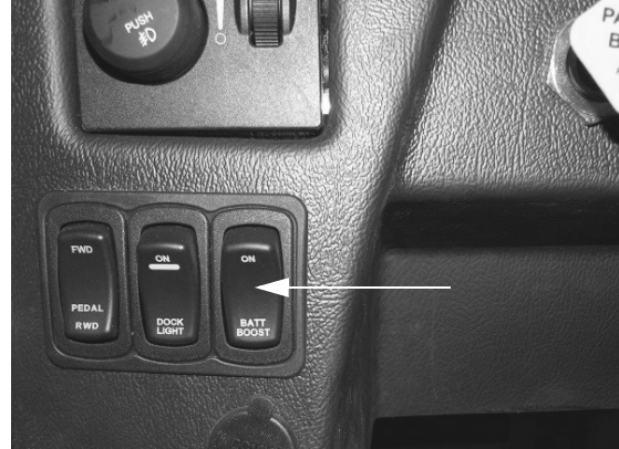
Battery Boost Switch (Located on dash)
