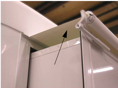
Slideout Cover-Awning -Typical View
