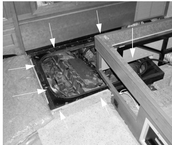
Step Cover Screw Locations (Shown with Metal Engine Covers removed) -Typical installation shown
