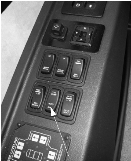
Tag Axle Switch (Located on the driver side trim panel) -Typical View
