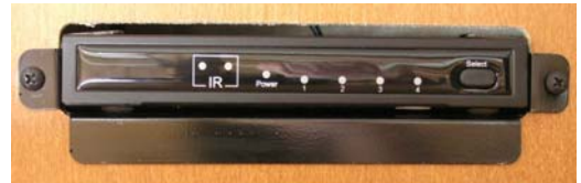
Secondary Source Selector (Located near each TV)
