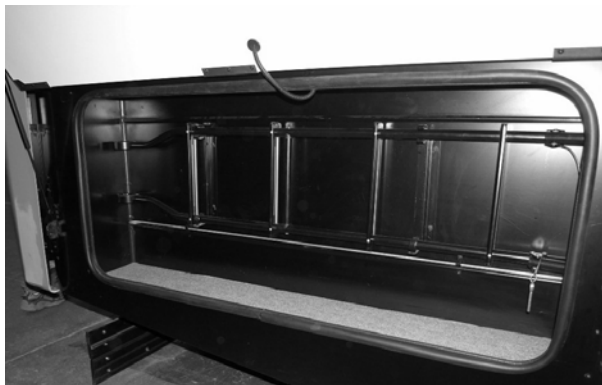
Roof Ladder Extension (Located in passenger rear compartment) -Typical View
