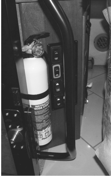
Fire Extinguisher (Located near entrance door) -Typical installation shown
