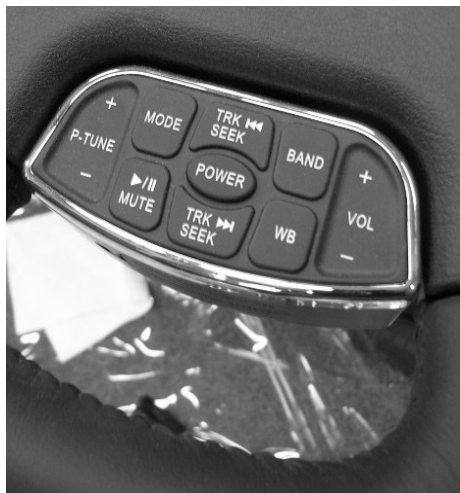
Steering Wheel Radio Remote Control
