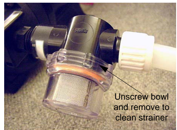
Water Pump Strainer -Typical View
