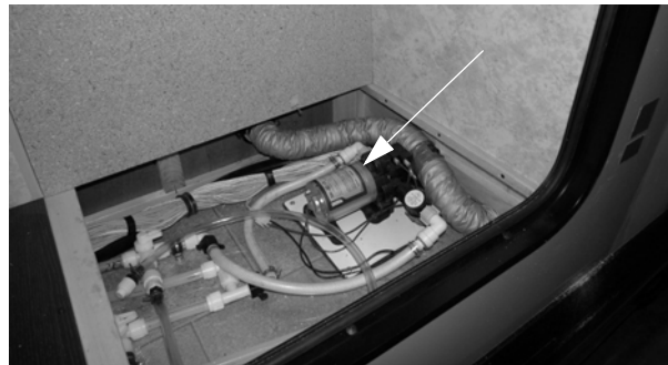
Water Pump (Located beneath removable access panel in passenger rear compartment) -Model 24M shown
