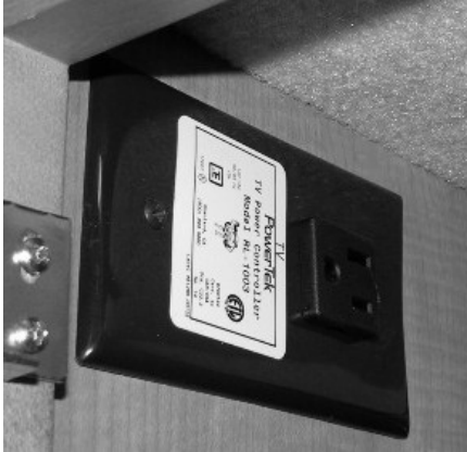
Front TV Ignition Switch Interlock -Typical View
