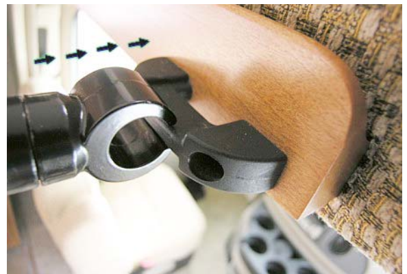
Attaching Bunk Ladder
