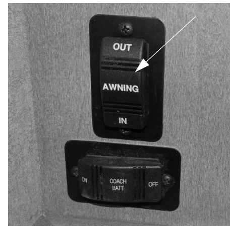
Power Awning Switch (Located near entrance door) -Typical View
