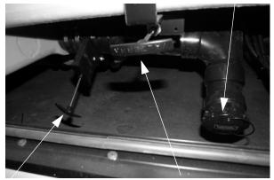
1st - Pull Black Waste Tank Drain valve to drain black water (sewage) tank then close. 2nd - Pull Gray Waste Tank Drain valve to drain gray water (sink/ shower) tank then close.
