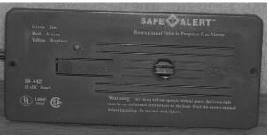
Propane Gas Leak Detector
