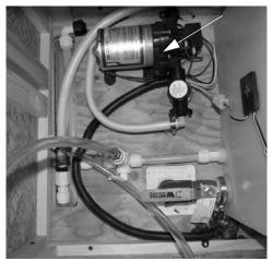
Water Pump (Located beneath bed lift mattress to expose access hole) -Typical View
