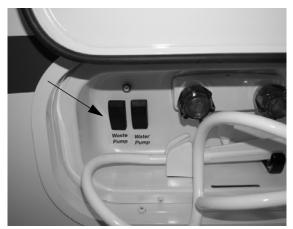
Waste Pump Switch (Located near exterior shower) -Typical View
