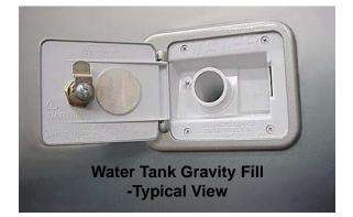
Insert hose into fill opening and turn water supply on. Tank is full when water flows from tank vent tube beneath coach.
