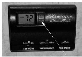
Temp SelectorPress up or down to select temperature
