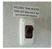
Holding Tank Heater Switch (Located near monitor panel) -Typical View
