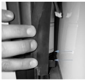
• Ensure slideout motor is disengaged approximately 1/2" from base.
