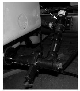
Waste Pump (Located on driver side of coach behind rear wheel) -Typical View
