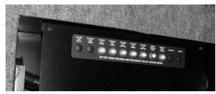
Chassis and House 12V Breakers (Located in passenger side compartment) -Typical View \* Shown with cover removed
