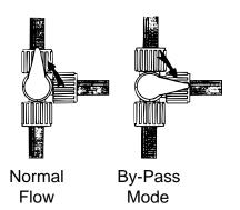
Leave Water Heater Bypass valve handle in NORMAL FLOW position if draining water and blowing out waterlines. Place in BYPASS position ONLY when using antifreeze solution in waterlines.
