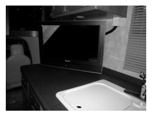
3. Rotate TV back to center position and press straight back towards wall. You will hear a "click" when the TV is secured into locked position.
