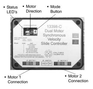
Slideout Control Panel (Located in passenger side compartment)
