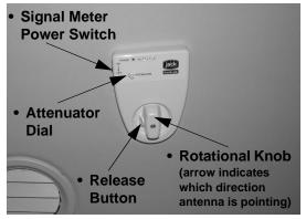
Digital Antenna Signal Meter (Located on ceiling)
