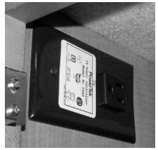
Front TV Ignition Switch Interlock -Typical View
