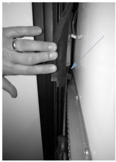
Slideout Motor (Located behind slideout wipe seal)
