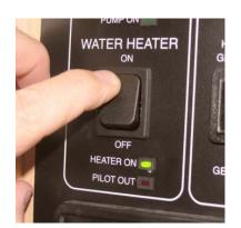
Gas Water Heater Switch (Located on Systems Monitor Panel)
