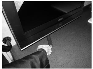
2. Pull the TV out and pivot to desired position.
