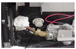
Water Heater Drain Plug (Remove with socket)
