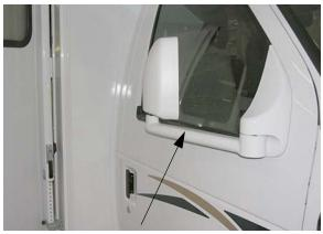
• The mirrors can be folded back against the cab doors, if needed.
