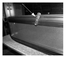
• Pull out the lever on the crank-out handle and begin cranking out the window counter-clockwise to the position desired.
