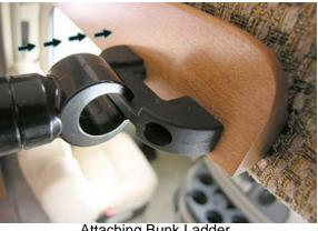
Attaching Bunk Ladder •Lift ladder horizontally •Slide C-shaped retainer ends at top of ladder onto brackets at rear edge of mattress.
