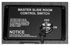
Master Slideout Room Keylock (Located near interior slideout control switches)
