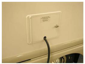
• Route power cord through passage and close door while shoreline is connected to outlet.
