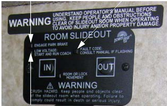
Low Voltage Indicator
