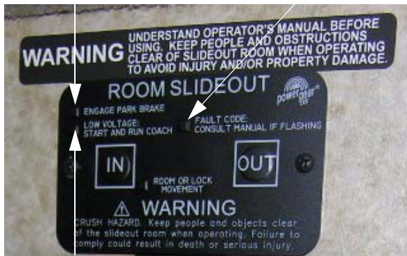
Low Voltage Indicator
