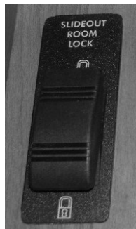
Slideout Room Travel Lock (Your model may be equipped with one or more types) -Typical View
