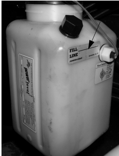
Hydraulic Oil Reservoir -Typical View
