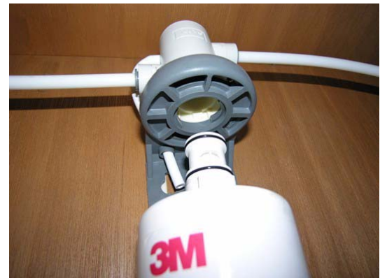
Insert new filter up into filter socket – Press and twist 1/4-turn clockwise (to the right).
