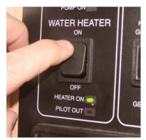
Gas Water Heater Switch (on Systems Monitor Panel)
