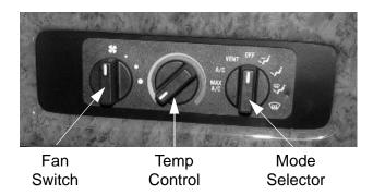
*NOTE:* The dash air conditioner/heater is not designed to heat and cool the entire interior of the coach, but is intended only to provide heating and cooling for the cab area.
