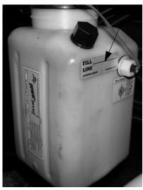
Hydraulic Oil Reservoir (Power Gear systems only) -Typical View
