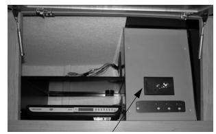
TV Signal Amplifier Power Switch (Typical View)
