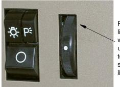
Roll panel light dimmer wheel upward fully to turn driver side map light on.
