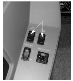
12-Volt Front Drop-Down Solar/Night Shade Switches (Typical View)
