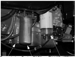
TransmissionEngine Oil FilterDiesel Fuel/WaterFluid Filter(Typical)Separator Filter(Typical)(Typical)
