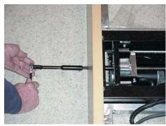
3. The slotted end of the tool must engage with the pin in the endshaft on the slideout gear assembly. See arrow in close-up detail.
