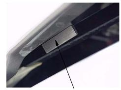
Squeeze latch handles toward hood panel and raise hood into open position
