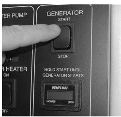
Generator Switch and Hourmeter (Located on monitor panel) -Typical View
