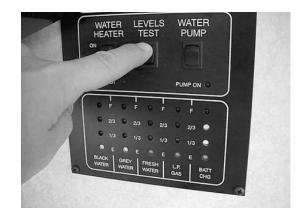
The approximate fluid levels are measured by electronic sensors on the sides of the tanks. There is generally more fluid in a tank than indicated on the monitor panel.
