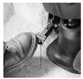
Press pedal to adjust steering wheel tilt
