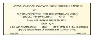
If any weight exceeding 45.4 kg (100 lbs.) is added to your coach between final vehicle certification and first retail sale, the occupant and cargo carrying capacity must be corrected and a label similar to the one shown below will be affixed inside your coach.
