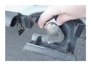
2. Swivel the cover section aside to reveal cord notch.
