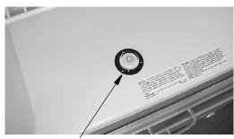
Place bubble level in bottom of refrigerator
