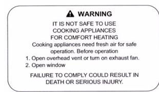
Unlike homes, the amount of oxygen supply is limited due to the size of the recreational vehicle, and proper ventilation when using the cooking appliances avoids dangers of asphyxiation.
