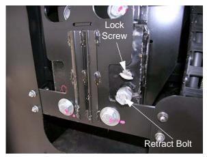
After loosening the lock screws, fit the ratchet wrench onto the bolt head and begin cranking clockwise slowly a few turns, then alternate to the other side for a few turns.
