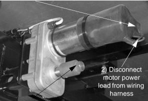
Use 3/4"socket on gearbox shaft. Crank both sides equally to avoid wedging
