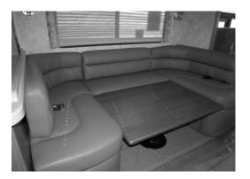
3. Secure both latches on the table leg to lock in lowered position.
