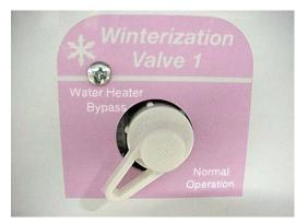
Leave bypass valve handle in NORMAL FLOW position if draining water and blowing out waterlines. Place in BYPASS position ONLY when using antifreeze solution in waterlines.
