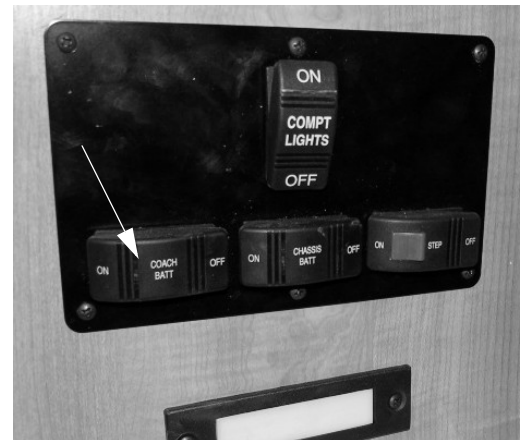
Auxiliary Battery Switch - Typical (Near Entrance Door)
