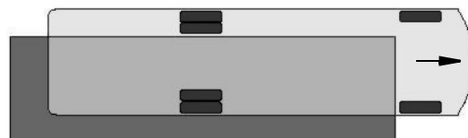
Weighing Right Rear Corner
