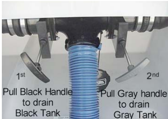
Holding Tank Dump Valves (Typical)
