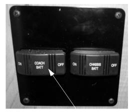
Auxiliary Battery Switch - Typical (Near Entrance Door)
