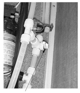
Water Heater Bypass Valve (Typical)
