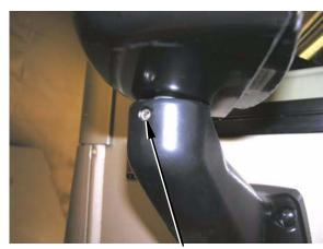
Mirror Head Pivot Lock Loosen Allen head set screw to pivot mirror head.\* (Torque 75-100 in/lbs)
