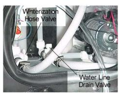
Winterization and Water Line Drain Valves - typical
