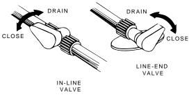
Water Line Drain Valve (Typical)
