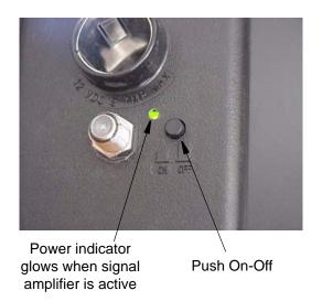
TV Signal Amplifier Power Switch (with 12-volt outlet and coaxial jack on wall plate in front overhead entertainment compartment)
