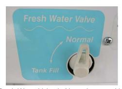
Fresh Water Valve in Normal use position (located in water service center)
