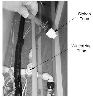
Winterization Valve beneath rear bed Model 30B shown
