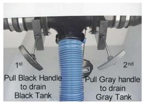
Holding Tank Dump Valves (Typical)
