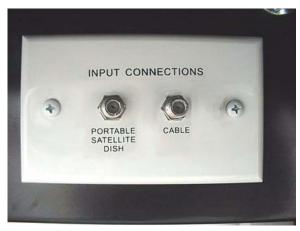
Satellite Dish and Cable TV Input (Hook-up) Connections (in Utility Compartment)
