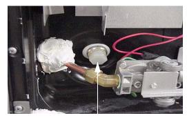
Water Heater Drain Plug (Remove with socket)
