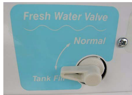
Fresh Water Valve in Tank Fill position (located in water service center)
