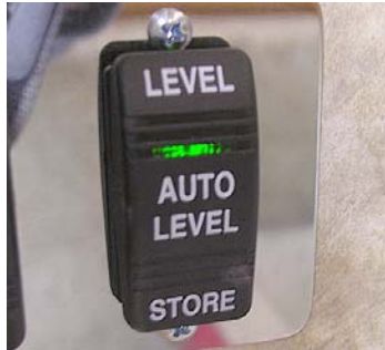
Auto Level Switch (Located inside entrance door)
