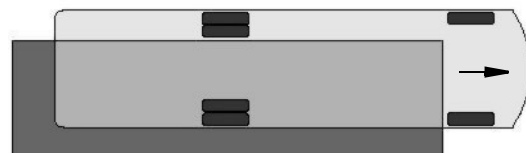
Weighing Right Rear Corner
