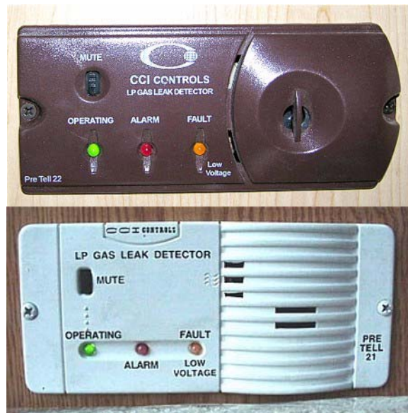
Propane Gas Leak Detectors (Typical)
