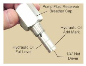
NOTE: Overfilling the hydraulic reservoir can cause leakage of oil through the breather cap.
