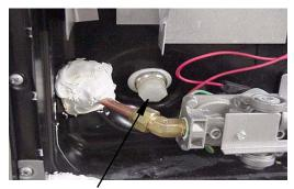
Water Heater Drain Plug Remove with socket.
