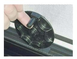
If the window will not open after three or more full turns of the knob, the glass may be stuck to the sealing gasket. Go to the outside of the coach
