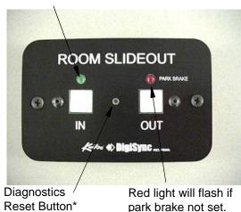
\*Not equipped on single mechanism systems
