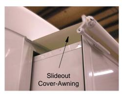
Also, freezing rain and snow can prevent the slideout cover-awning (if equipped) from closing and may cause damage to the cover-awning, slideout room, weather seals and mechanisms.
