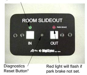
\*Not equipped on single mechanism systems
