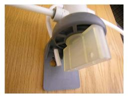
2. Remove the filter canister from the full-coach water filtration system in the water center compartment (if equipped) and discard the filter cartridge. (If your coach is not equipped with a full-coach water filtration system, proceed to the next numbered step.)
