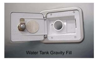
Insert hose into fill opening and turn water supply on. Tank is full when water flows from tank vent tube beneath coach.
