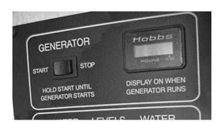
Refer to the hourmeter to determine when periodic maintenance is due and to record services which have been performed.
