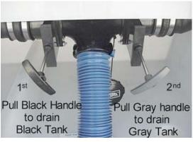
Holding Tank Dump Valves (Typical)
