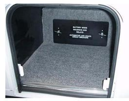
Chassis and House 12V Breakers in exterior storage compartment (remove cover to access)
