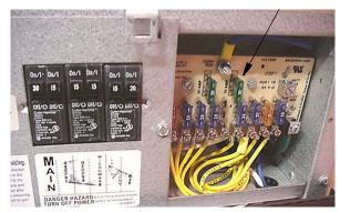
The fuse panel accepts only blade type plug-in fuses. Always replace fuses with those of the same amperage rating.
