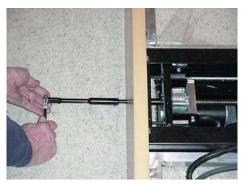
• The slotted end of the tool must engage with the pin in the endshaft on the slideout gear assembly. See arrow in close-up detail.
