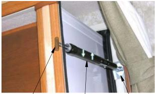
Place T-shaped rod end against back side of slideout frame
