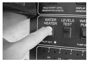
The "Pilot Out" light will glow for about 10-15 seconds, then it will go out. The "Heater On" indicator will remain lit. • If the "Pilot Out" light comes on during propane operation, it means that the burner has gone into "lockout" mode and must be restarted. If this happens, turn the Water Heater switch off for about 5 minutes, then turn it back on.
