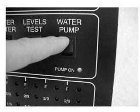
(Some models may also have a pump switch in the water system compartment on the outside of the coach.)
