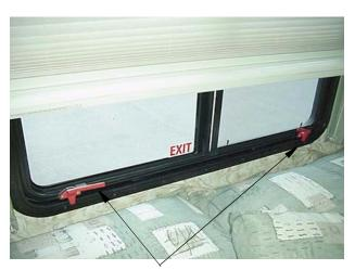
Escape Window - Lift latch handles upward to open.
