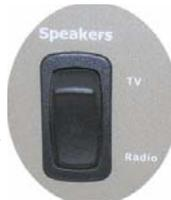
*NOTE: The Aux. Battery Disconnect switch must also be on while listening to Theater Sound because the audio relay is powered by house batteries. If the Aux Batt switch is off, the speakers will not emit any sound.*
