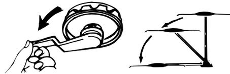
Turn elevating crank (counterclockwise) in "DOWN" direction until resistance is noted (about 13 turns). Antenna is now locked in travel position. Turn amplifier power switch "OFF".
