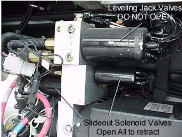
Leveling/Slideout System Hydraulic Pump
