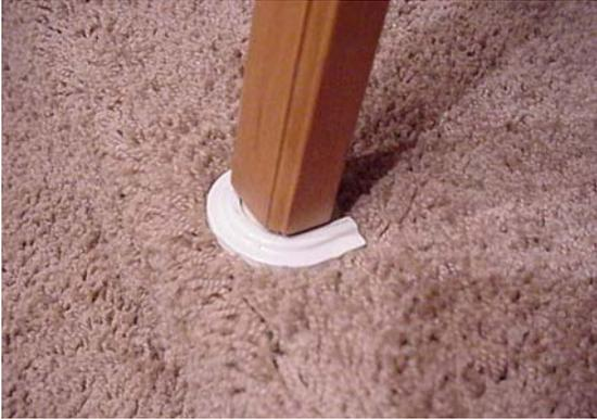
3. Refit the seat support 'bumpers' onto the seat frame.
