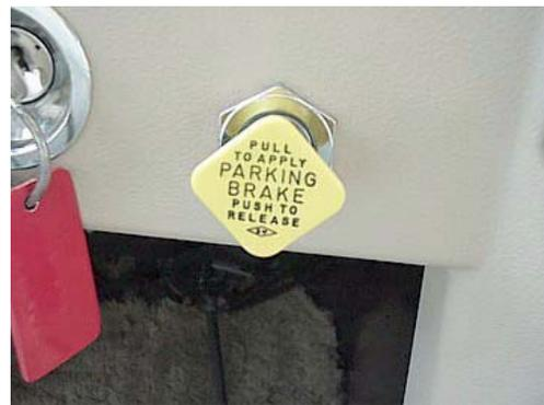
*Note: Never drive your vehicle with the parking brake set. It will reduce parking brake effectiveness and cause excessive wear.*
