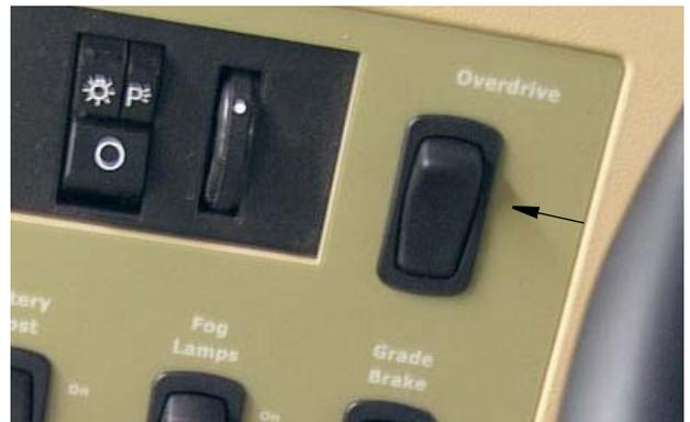
When this switch is ON, the transmission will automatically shift to the overdrive gear whenever possible for greatest fuel economy.
