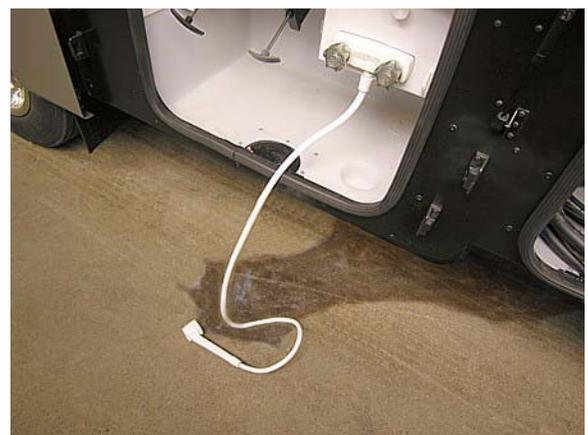
Using Exterior Shower to drain waterline
