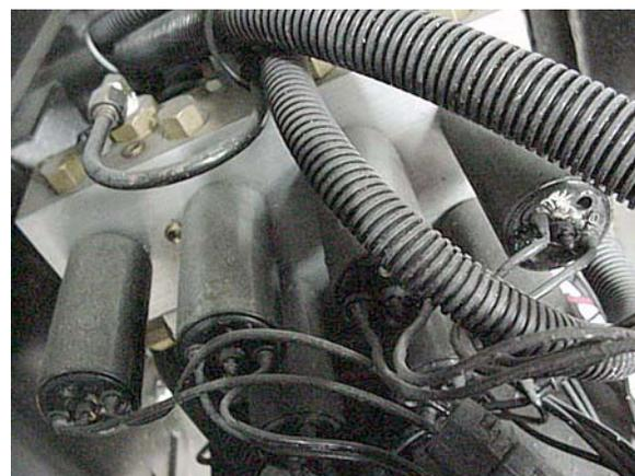
Leveling/Slideout System Hydraulic Pump
