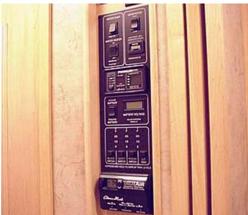
At the touch of a button this panel can display the fresh water and holding tank levels, propane gas tank level, plus the battery and house battery condition. You can start the electric generator or turn on the water pump and water heater. Indicator lights tell you if the water pump is on or if the water heater pilot light is out.
