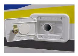
Water Tank Gravity Fill
