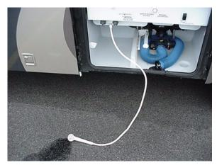
4. Turn on water pump and open all sink faucets and shower head knobs. Leave open after water stops flowing.
