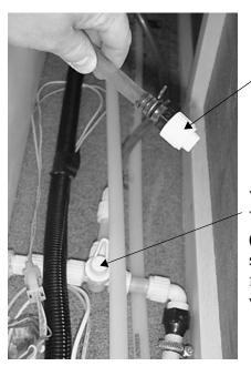
Siphon Tube (insert into container of RV water system antifreeze)
