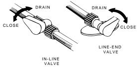
Water Drain Valves (typical)
