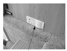
LP Gas Leak Detector
