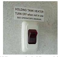
DO NOT operate the holding tank heaters unless you are providing a supplemental 12-volt power source to recharge the house batteries.
