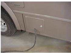
The three-prong power cord is designed to ground the electrical system through the receptacle. It is also designed to carry the amperage output of most campground outlets. If the electrical receptacle to be used is designed to mate with the three prongs on the power cord plug, the electrical connection can be expected to carry rated load.
