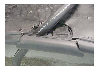
3. Route the cord through the notch, flip the hatch back up into place and close the compartment door.
