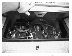
Remove step cover to access batteries
