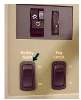
Battery Boost Switch If engine battery is dead, press and hold while turning ignition key for emergency starting power.
