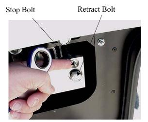
After loosening the lock screws, fit the ratchet wrench onto the bolt head and begin cranking clockwise slowly a few turns, then alternate to the other side for a few turns.
