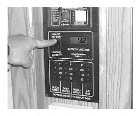
The LCD display will show the current battery voltage to the nearest tenth of a volt.
