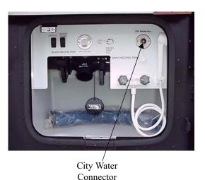
3. Turn water tank fill valve to CITY FILL position.
