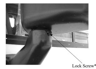
Side Mirror Loosen screw to make coarse adjustment
