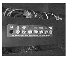
Automotive Fuse/Breaker Panel (Behind Panel on Top Step)
