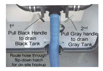
When using a sewer hook-up, keep the dump valves closed until a tank becomes full or when preparing to leave the site. This keeps the solids in suspension, allowing them to be carried out with the liquids when the dump valve is opened. If the valve is left open, the liquids will drain off,
