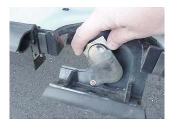
2. Swivel the cover section aside to reveal cord notch.
