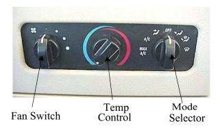
**Fan Switch -** Smallest dot is lowest air movement; Largest dot is maximum air movement. Fan will run at set speed when mode knob is in any position except Off. When mode knob is set to Off, the fan will not run.
