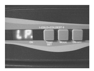
To operate in the MANUAL mode, press and hold the MODE button until AUTO disappears and the desired operating mode is displayed. If the power source is interrupted while operating in the MANUAL mode, a diagnostic code will appear, an alarm will sound, and the refrigerator will cease operation. For corrective actions, refer to the *Diagnostic Codes and Their Meaning* on page 10 of the refrigerator Operator's Guide in your Owner InfoCase.
