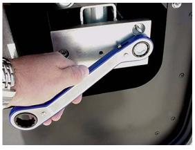
Crank the wrench(es) clockwise slowly, until the room is fully retracted. Allow about 10 minutes to crank room in fully.
