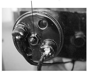
Slideout Room Solenoid Valve
