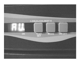
The ON/OFF button turns the refrigerator on or off. If the button is pressed, it will turn the refrigerator on and set the mode to auto. When the refrigerator is on, pressing this button for 2 seconds will turn the refrigerator off.
