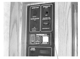
Generator Switch and Hourmeter
