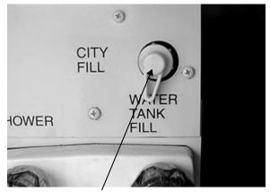
Turn tank fill valve to WATER TANK FILL position.
