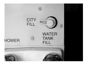
NOTE: Because city water pressure varies from location to location, we recommend using an in-line water pressure regulator to prevent damage to any components, connections and seals in your fresh water system.
