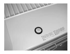
Place bubble level in bottom of refrigerator
