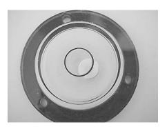
If over 1/2 of the bubble is inside the circle in any direction, the coach is level enough for continuous operation of the refrigerator while parked.
