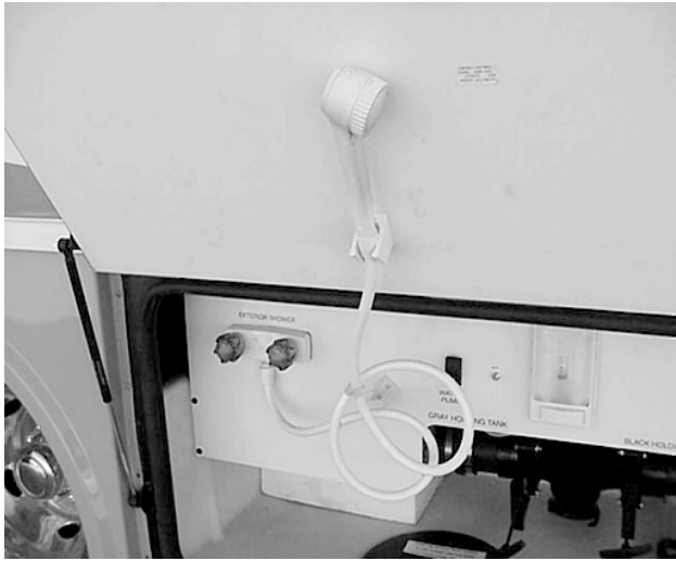
Exterior Shower/Wash Station (Typical)
