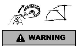
Never allow the antenna to touch electrical power lines or any other electrical wires. **Rotating Antenna** - Make sure antenna is in the "UP" position. Pull down on rotating knob until it disengages ceiling plate and rotate for best picture and sound on TV set.
