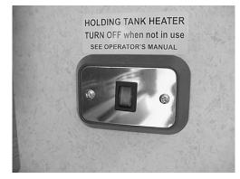
Do Not Operate the holding tank heaters unless you are providing a supplemental 12-volt power source to recharge the house batteries. This means either the shoreline cord must be plugged into a 110-volt source, or the auxiliary
