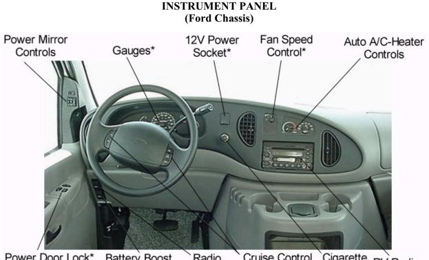
Power Door Lock\* Battery Boost Radio Cruise Control Cigarette RV Radio & Window Buttons Switch Power Switch Buttons Lighter
