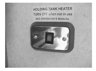
NOTE: The holding tank heater pads are electrical resistance type heating elements. This type of heating element typically uses a large amount of current while operating. If the tank heaters are used without a recharging source, they will drain the house batteries in a relatively short period. Typically, the batteries would not support overnight heating without a supplemental charging source.
