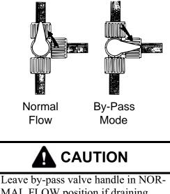
MAL FLOW position if draining water and blowing out water lines. Place in BYPASS position ONLY when using antifreeze solution in water lines.
