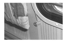
*To loosen the tension*, unwrap the guide cords from the spools one turn at a time until desired tension is achieved.
