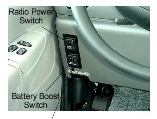
If engine battery is dead, press and hold while turning key for emergency starting power.
