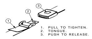
**Adjustment:** To lengthen belt, swivel tongue at a right angle to belt and pull to desired length. To shorten, pull loose end of belt.
