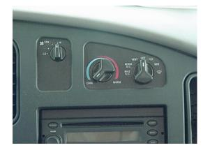
*NOTE:* The automotive air conditioner is not designed to cool the entire interior of the motor home, but is intended to cool the driver's compartment only.
