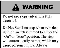
remember to retract the step before moving the vehicle.
