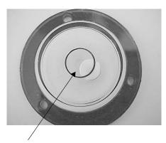
If over 1/2 of the bubble is inside the circle in any direction, the coach is level enough for continuous operation of the refrigerator while parked.
