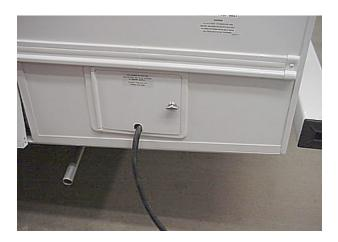
The three-prong power cord is designed to ground the electrical system through the receptacle. It is also designed to carry the amperage output of most campground outlets. If the electrical receptacle to be used is designed to mate with the three prongs on the power cord plug, the electrical connection can be expected to carry rated load. (See approximate power consumption table on page 6-5.)
