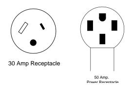
The optional 50-amp shoreline gives your coach extra current handling capacity. This allows you to run both roof air conditioning units at maximum (both compressors running) without fear of constantly tripping circuit breakers.
