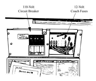
The fuse panel accepts only blade type plug-in fuses. Always replace fuses with those of the same amperage rating.
