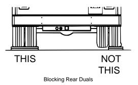
To provide extra firmness, you can place inexpensive mechanical jacks, jack stands or hydraulic "bottle" jacks under the frame to keep the coach from moving on the suspension springs while walking around inside the coach. These devices are not intended to lift the coach; only to hold it rigid and steady.
