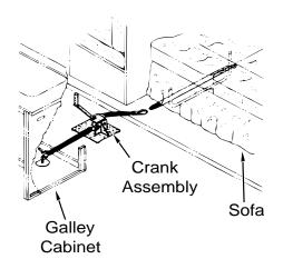
Model 34V - Fasten winch belt to bolt under galley sink as shown.
