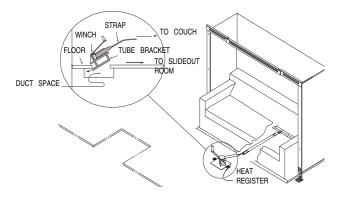
Model 33B - Remove floor register and insert crank assembly as shown.
