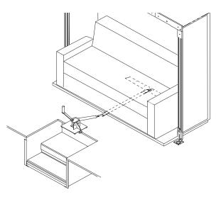
Model 35C & 37G - Winch hooks onto lip of top entrance step as shown.
