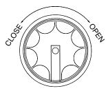
If the window will not open after three or more full turns of the knob, the glass may be stuck to the sealing gasket. Go to the outside of the coach and gently free the glass with your fingers. A periodic light dusting of talcum powder on the gasket should prevent this from recurring.
