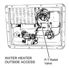
Normally there is an air gap at the top of the water heater tank which acts as a pressure buffer. In time, however, heated water may expand and fill this air gap, causing a slight increase in water pressure. This may cause the P-T valve to "weep" until the air gap is manually replaced.
