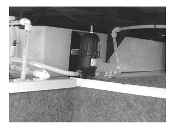
NOTE: The accumulator tank has a precharge pressure which must be **checked month***ly* and maintained at **20 psi** for the system to work properly.
