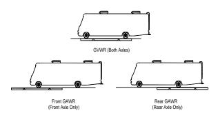
To determine the weight on either front or rear axle, drive that axle only onto the scale. Neither axle weight should exceed the corresponding maximum axle weight rating specified on the certification label.
