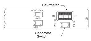
NOTE: While the generator is running it is normal for the hourmeter to make a periodic "ticking" sound.
