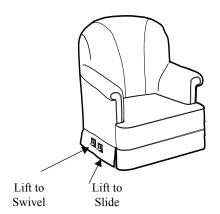
Swivel: Pull up on the swivel lever located on the side of the seat. The seat will lock into place whenever it reaches the center aisle facing position.
