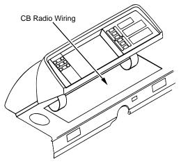
Look for a pair of wires, purple (+) and green (-), with connectors and flag labels, suspended from the wiring harness.
