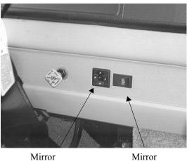
Mirror Adjustment Control Mirror Heat Switch
