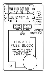
Automotive/Chassis Fuse Block and Breaker Panel
