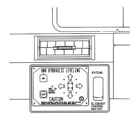
• Press slide-out switch and hold until room is fully extended, then release switch.
