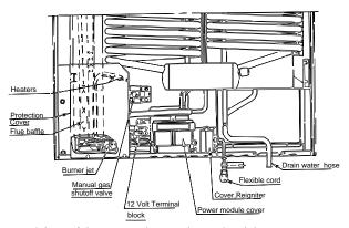
This refrigerator is equipped with an Automatic Energy Selector (AES) control system, which can automatically select the most suitable energy source which is available, either 120 Volt AC, or LP gas operation. The system can be set by the user to be fully automatic, or if desired, LP gas only. The refrigerator controls will work down to 9.6 volt DC.
