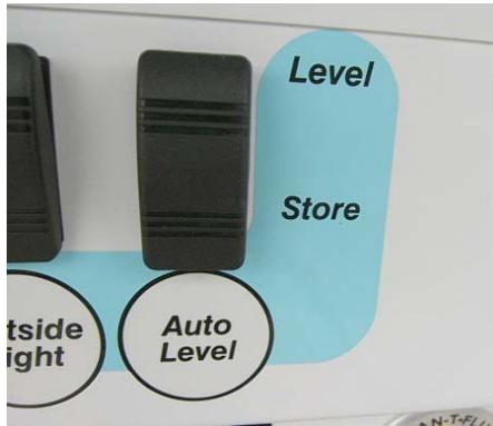
Auto Level Remote Switch (Located in the utility compartment) -Typical View
