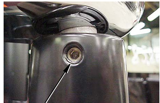
Allen Head Set Screw* (Torque screw to 75-100 in./lbs.)
