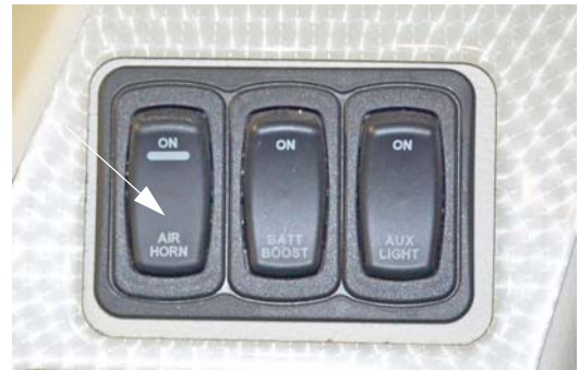
Air Horn Switch (Located on dash) -Typical View
