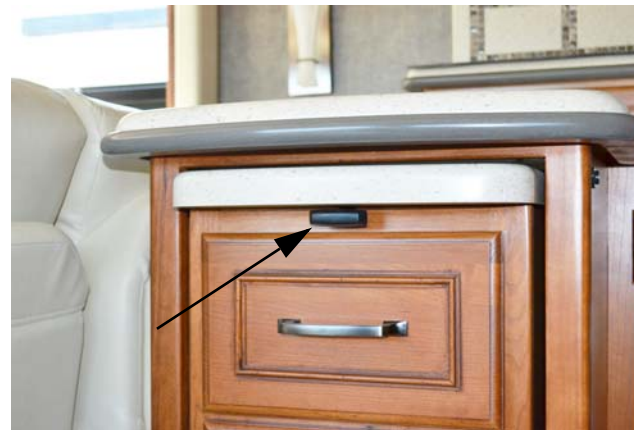
Countertop Extension Release Lever (Located underneath countertop extension lip) -Typical View
