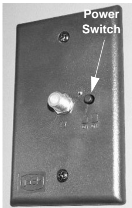
TV Signal Amplifier Power Switch (Located in overhead compartment above entrance door) -Typical View
