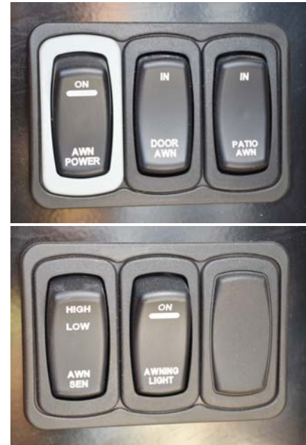
Awning Control Switches (Located near entrance door) -Typical View
