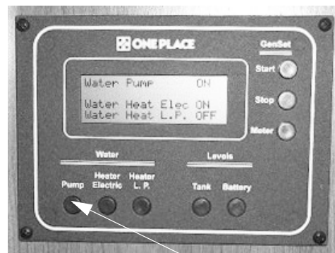
Water Pump Switch
