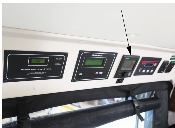
Water heater controls on Systems Monitor Panel *Model 59KL shown -Typical View
