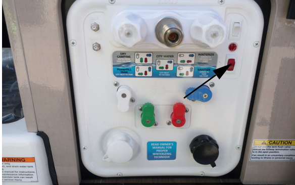
Exterior Utility Light Switch (Located in the Water Center Panel.) *Model 59KL Shown -Typical View
