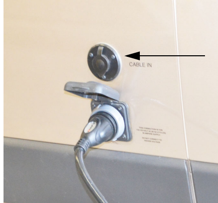
Cable TV Input Connection (Located on the left sidewall) *Model 59GL shown
