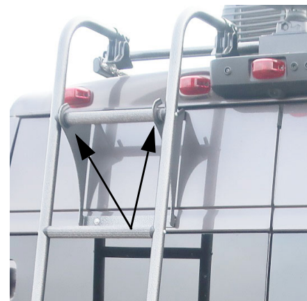
Ladder Storage Rungs -Typical View
