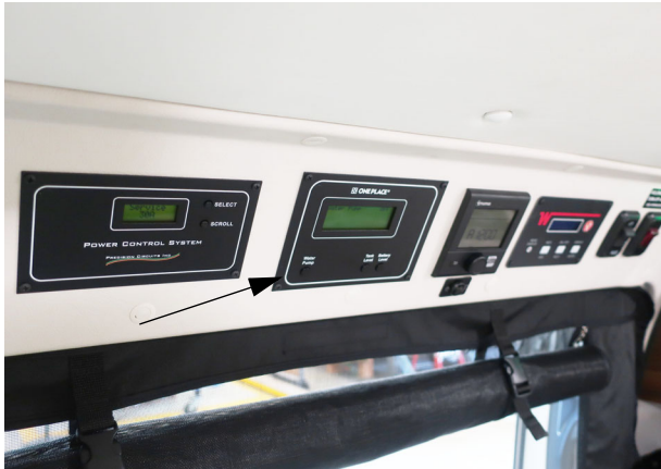
Water pump switch location on Systems Monitor Panel *Model 59KL shown -Typical View
