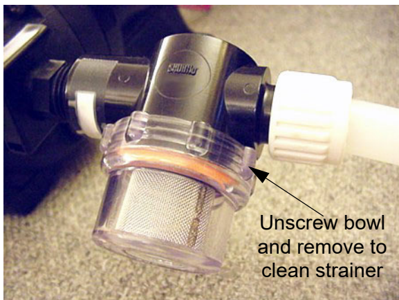
Water Pump Strainer -Typical View
