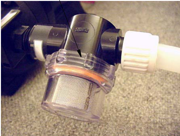
Water Pump Strainer in Water Service Center (typical)
