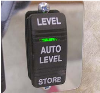
Auto Level Switch (Located inside entrance door)
