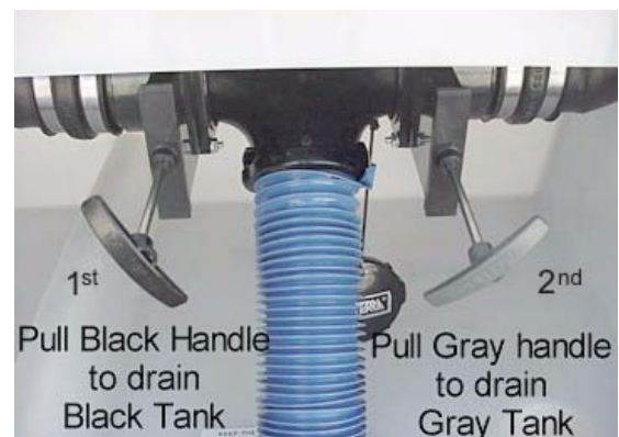
Holding Tank Valves (Typical)
