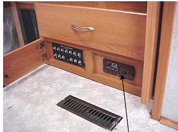
LP Gas Alarm
