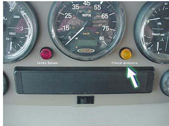
“Check Antenna” Light
