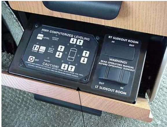
Leveling System Control Panel
