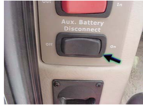
Aux. Batt. Switch (on entry panel)
