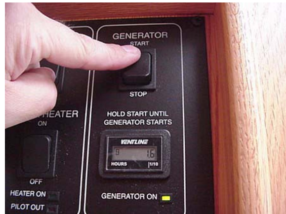
Generator Switch and Hourmeter
