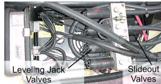
Slideout Pump beneath Entry Step
