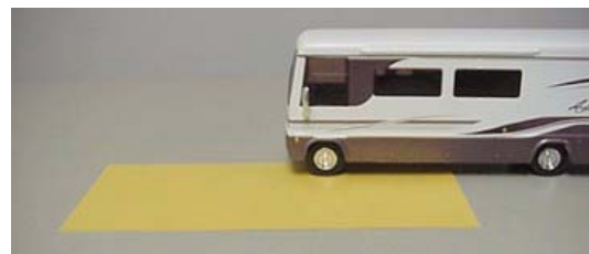
Weighing Left Front ‘Corner’
