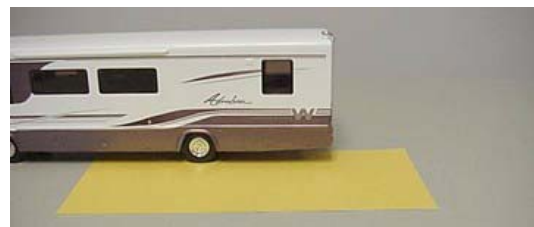
Weighing Left Rear ‘Corner’
