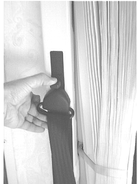
Press lever to adjust shoulder belt height
