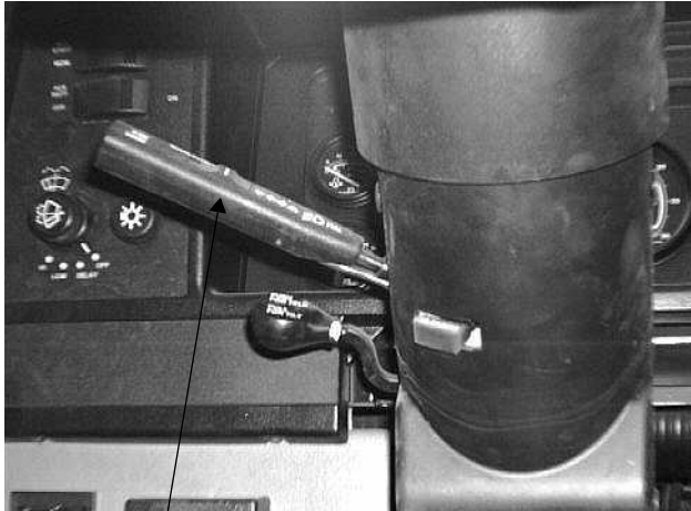
Multifunction Lever Signals/Hi-Lo Beams/Cruise
