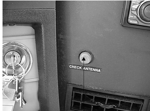
“Check Antenna” Light
