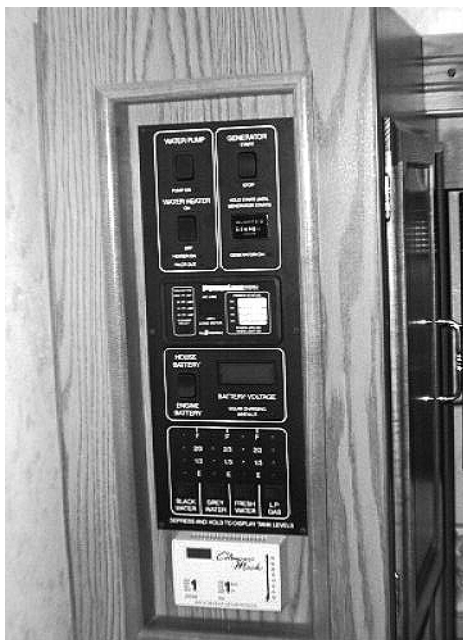
One Place Monitor Panel
