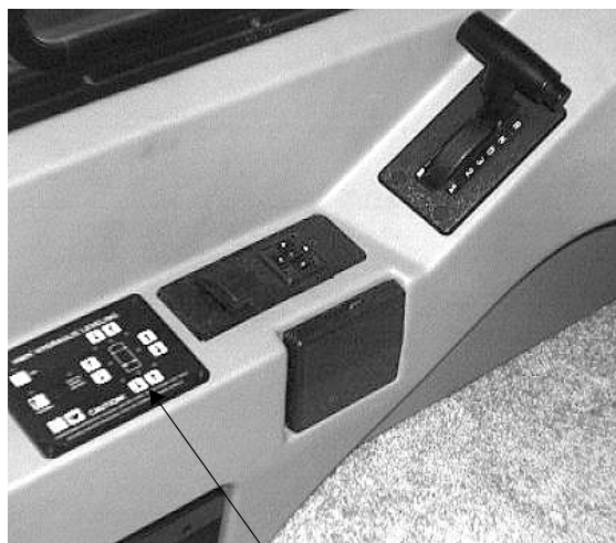
Leveling System Control Panel
