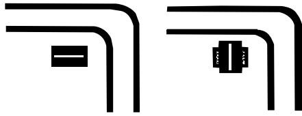
CLOSE OPEN Refrigerator Access Door Latches
