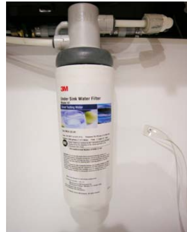
Galley Cold Water Faucet/ Ice Maker Filter Assembly (Located below galley sink) -Typical View
