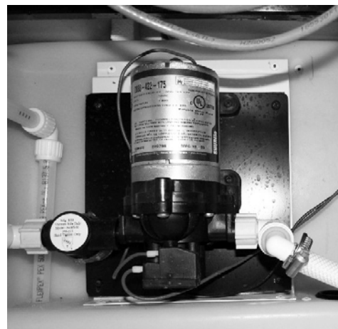
Water Pump (Located inside driver side compartment behind rear wheel) -Typical installation shown
