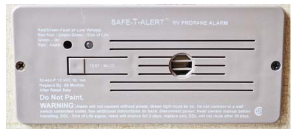
Propane Gas Leak Detector
