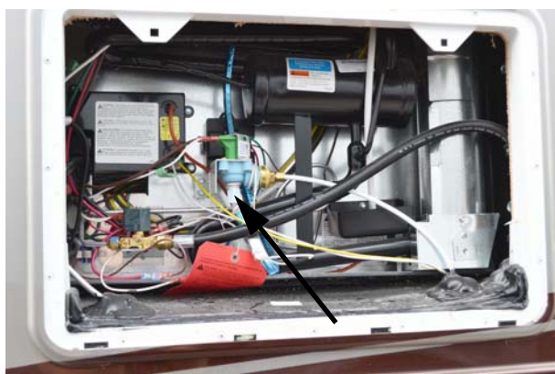
Ice Maker Water Supply Connection -Typical View
