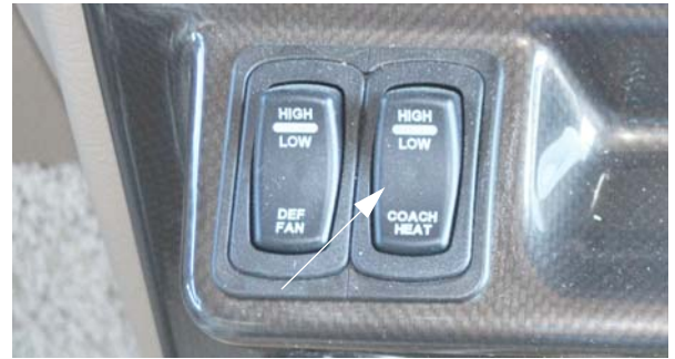
Coach Heat Switch (Located on dash) -Typical View
