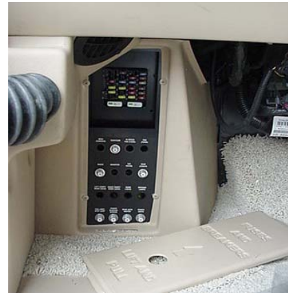
Automotive 12-Volt Circuit Breakers and Fuses (Located beneath left end of dash) -Typical View
