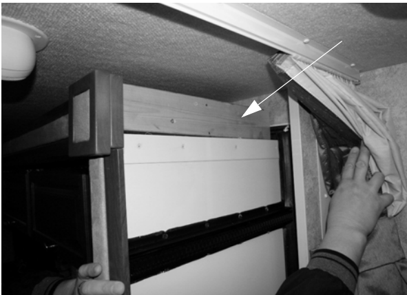
Slideout Travel Support -Typical installation shown
