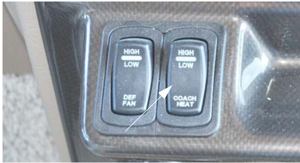
Coach Heat Switch (Located on dash) -Typical View
