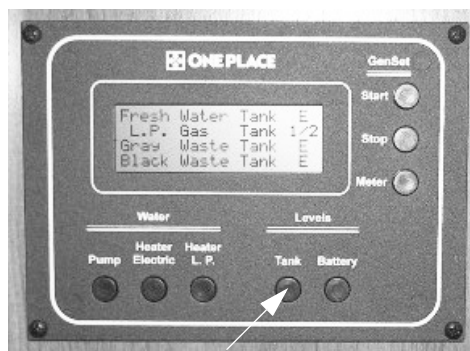
Tank Levels Switch
