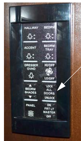
Power Door Locks - All Doors -Typical View
