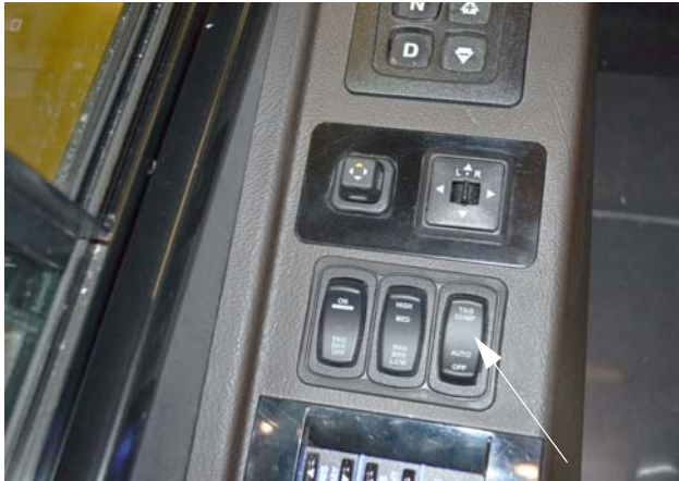
Tag Axle Switch (Located on the driver side trim panel) -Typical View
