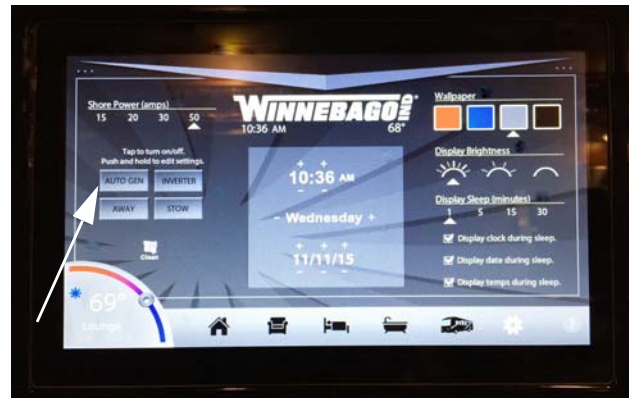
Generator Switch (Located on touch tablet “Utilities” screen)
