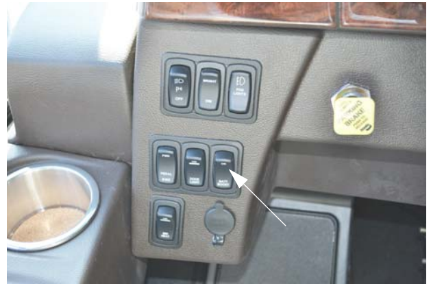
Battery Boost Switch (Located on dash)
