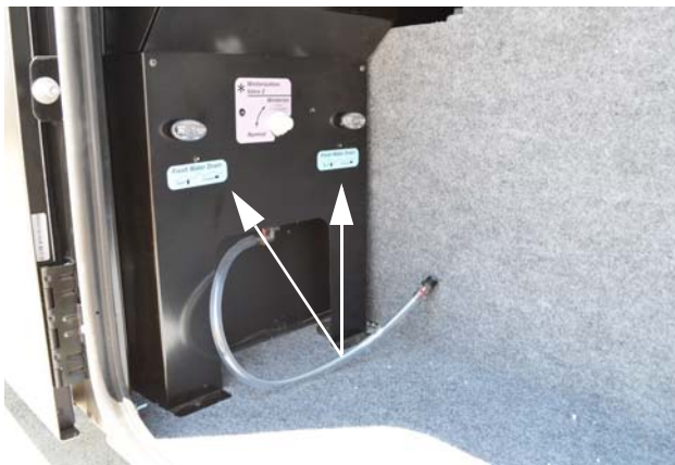
Waterline Drain Valves (Located in the third passenger side compartment) -Typical View
