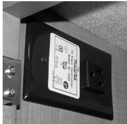
Front TV Ignition Switch Interlock -Typical View
