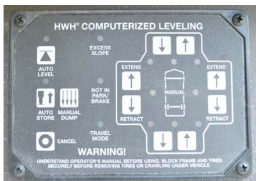
Hydraulic Leveling System Control Pad (Located on driver side trim panel) -Typical View
