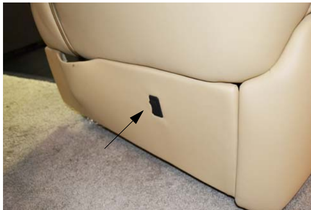
Power Lumbar Switch (Located on outboard side of seat) -Typical View
