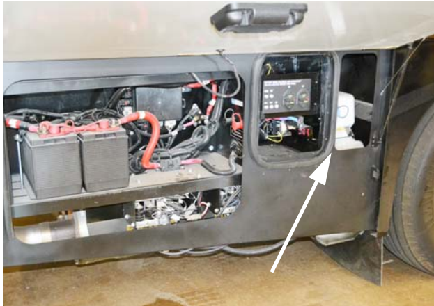
Diesel Exhaust Fluid Fill Tank *with Side Radiator (Located in passenger side compartment behind the rear wheel) -Typical View
