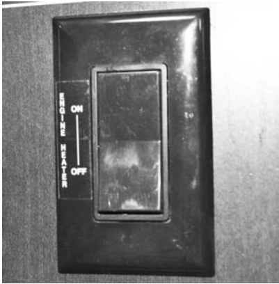
Diesel Engine Heater Switch (Located near monitor panel) -If Equipped
