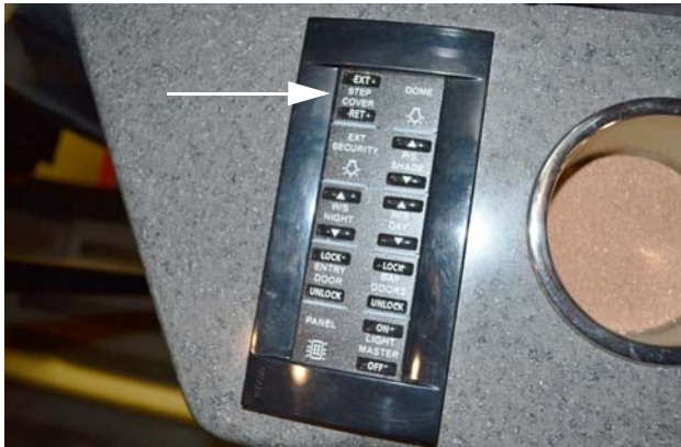
Step Cover Switch (Located on passenger side cabinet) -Typical View
