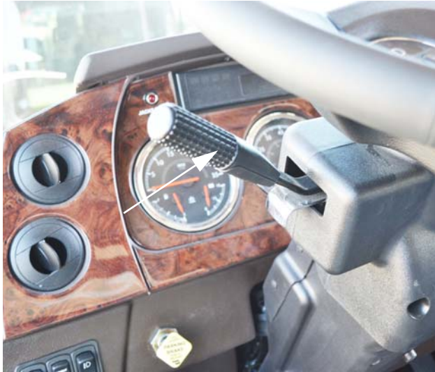
Turn Signals/High-Low Beams (Typical View - your coach may differ depending on model)
