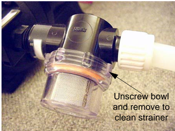
Water Pump Strainer -Typical View
