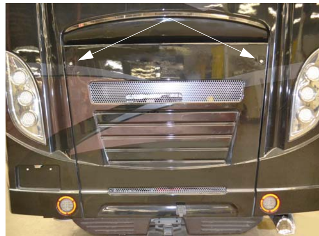
Engine Service Access Grille (Release latches and swing grille out) -Typical View
