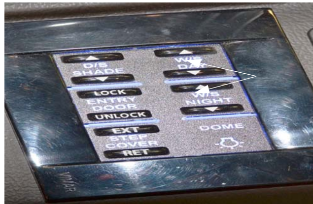
12-Volt Front Drop-Down Solar/Night Shade Switches (Located on driver side trim panel) -Typical View
