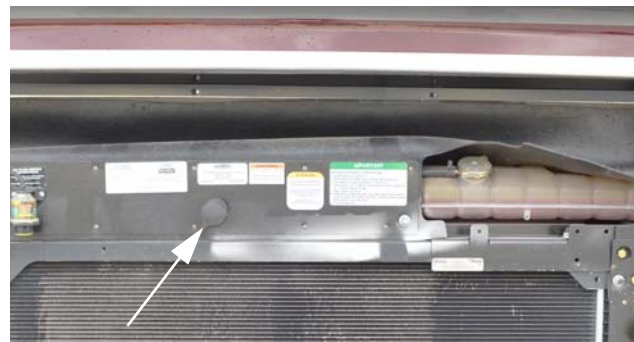
Diagnostic Plug (Located on rear engine compartment shroud) -Typical View
