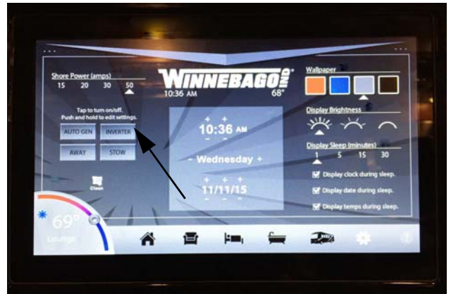
Inverter Power Switch (Located on touch tablet “Utilities” screen) Tap “Inverter” to turn on/off. • White text indicates ON. • Black text indicates OFF.
