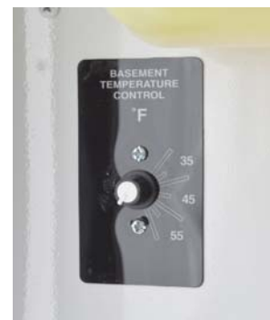
Basement Temperature Control (Located in driver side compartment) -If Equipped
