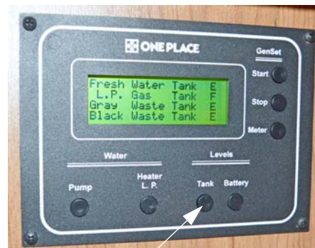
Tank Levels Switch
