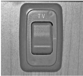
12-Volt TV Master Power Switch (Located in overhead cabinet or on a wall near the TV) -Typical installation shown
