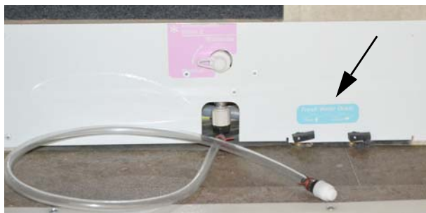
Waterline Drain Valve
