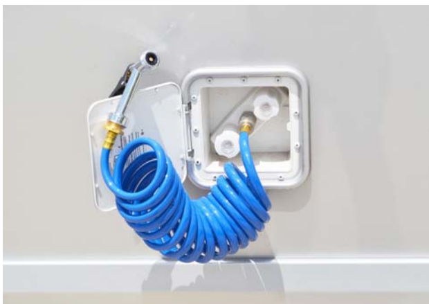
Exterior Shower/Wash Station (Typical)
