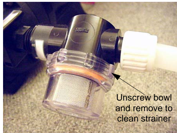
Water Pump Strainer -Typical View
