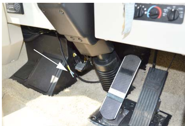
CB Power Wires -Typical View
