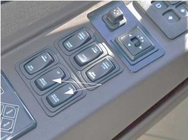
12-Volt Front Drop-Down Solar/Night Shade Switches (Located on driver side trim panel) -Typical View
