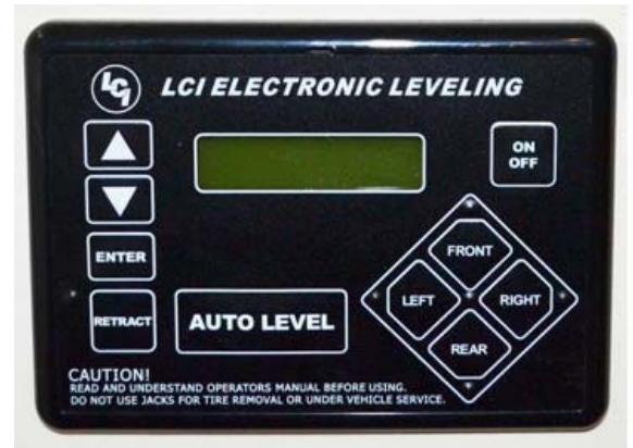
Leveling System Control Pad (Located on driver side trim panel)
