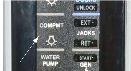
Compartment Lights Switch (Located near entrance door and/or inside a driver side compartment) -Typical View
