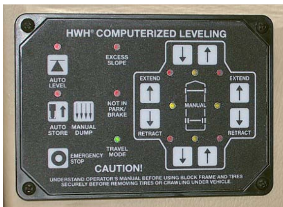
Leveling System Control Pad (Located on driver side trim panel)
