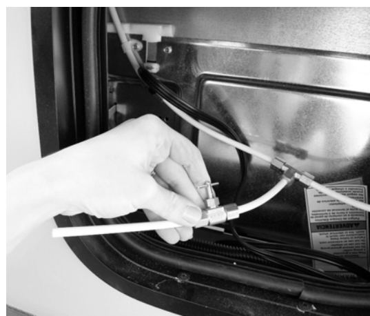
Ice Maker Winterization Drain Valve (Located in exterior Residential Refrigerator service compartment)
