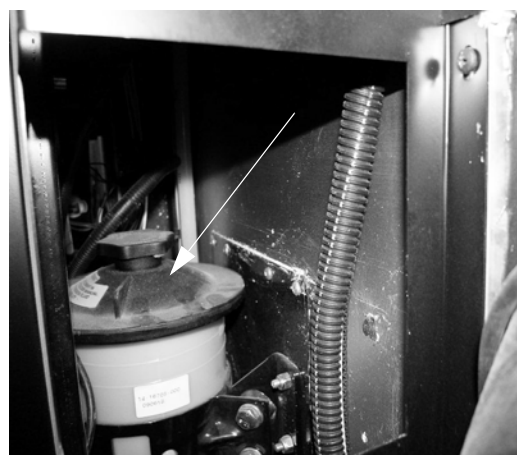
Power Steering Fluid Reservoir (Located in recessed area at LH side of rear engine service access grille) -Typical View
