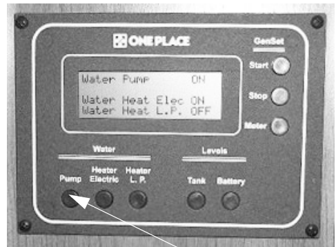
Water Pump Switch
