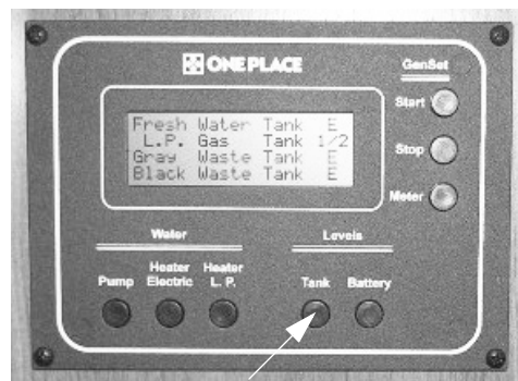
Tank Levels Switch
