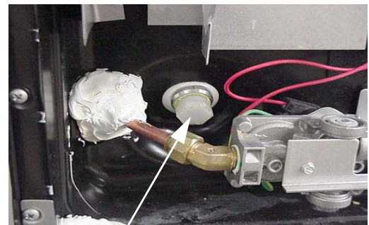
Water Heater Drain Plug (Remove with socket)
