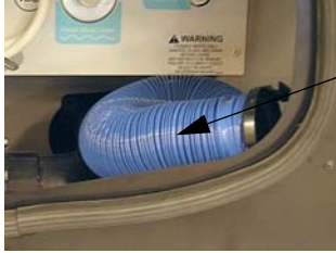
Sewage Drain Hose -Typical View
