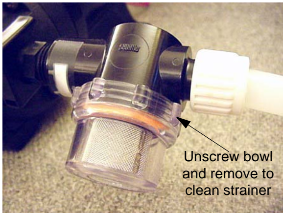
Water Pump Strainer -Typical View
