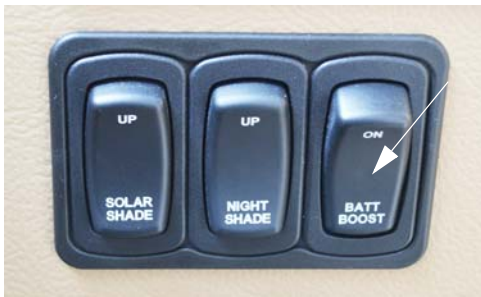
Battery Boost Switch (Located on dash)
