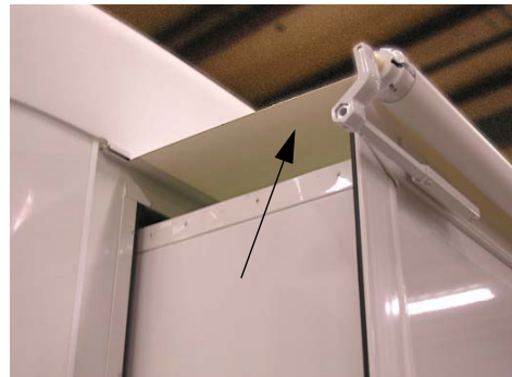
Slideout Cover-Awning -Typical View
