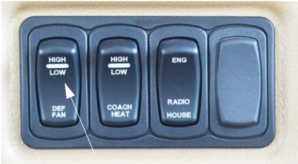
Defrost Fan Switch -Typical View
