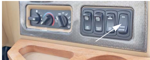
Radio Power Switch (Located on dash)
