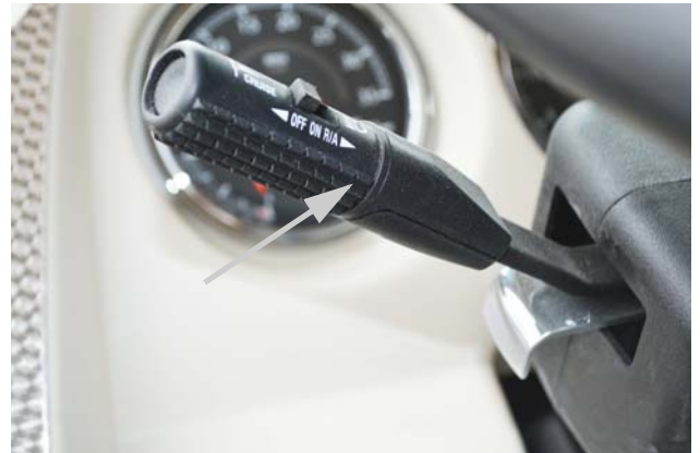
Turn Signals/High-Low Beams (Typical View - your coach may differ depending on model)
