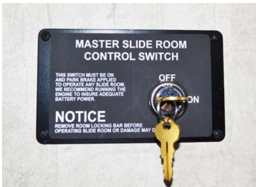
Master Slideout Room Keylock (Located near interior slideout control switches)
