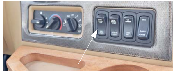
Defrost Fan Switch (Located on dash) -Typical View
