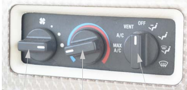
Blower Control Temp Control Mode Selector
