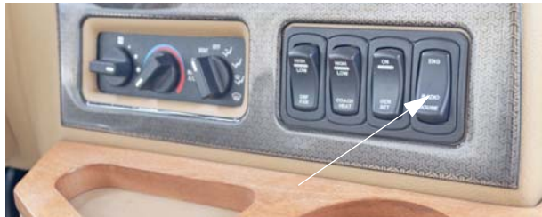
Radio Power Switch (Located on lower dash area)
