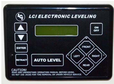
Leveling System Control Panel (Located on dash)
