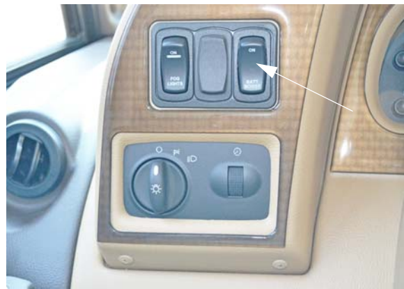
Battery Boost Switch (Located on dash) -Typical View
