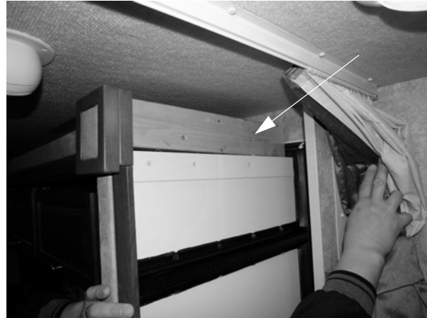
Slideout Travel Support -Typical installation shown
