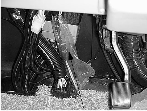
CB Power Wires (in plastic sheath)
