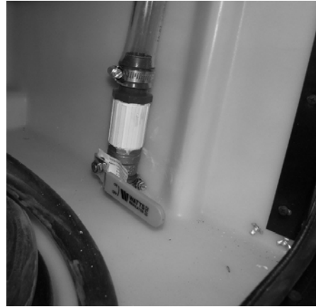
Water Tank Drain Valve -Typical installation shown
