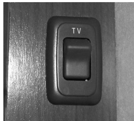
Bedroom TV 12-Volt Master Power Switch (Located on cabinet or wall near TV) -Typical installation shown
