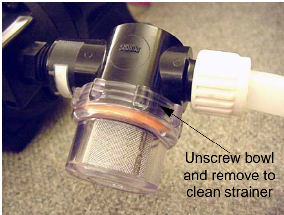
Water Pump Strainer -Typical View
