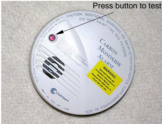
Carbon Monoxide Alarm
