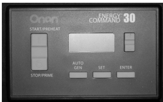
AGS Control Pad (Located near monitor panel)
