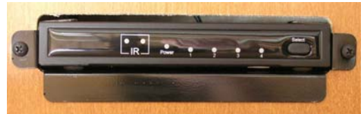
Secondary Source Selector (Located near each TV)
