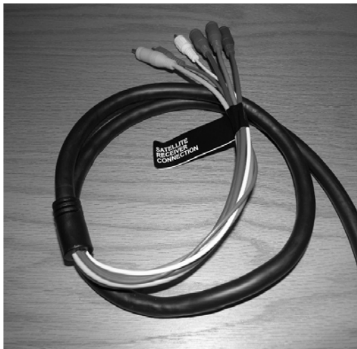
Audio/Video System Cables (Located in front overhead entertainment center cabinet)
