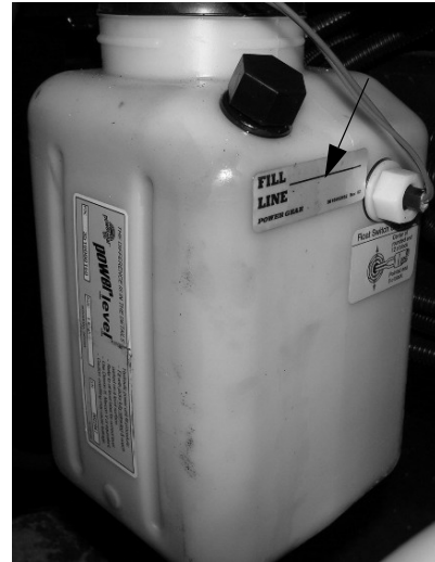
Hydraulic Oil Reservoir -Typical View
