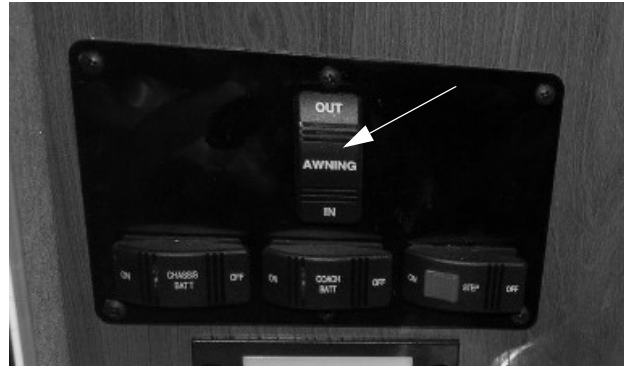
Power Awning Switch (Located near entrance door) -Typical View
