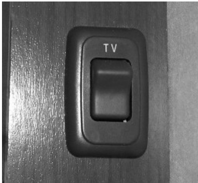
12-Volt Master Power Switch (Located in rear overhead cabinet or on a wall near the TV) -Typical View
