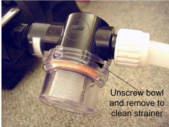
Water Pump Strainer -Typical View
