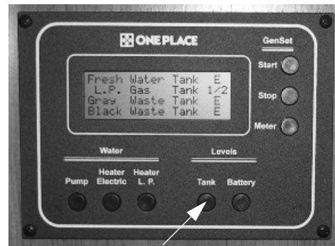
Tank Levels Switch
