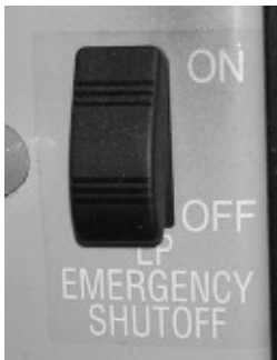
Main Tank Shutoff Switch (Located in driver side compartment) -Typical View
