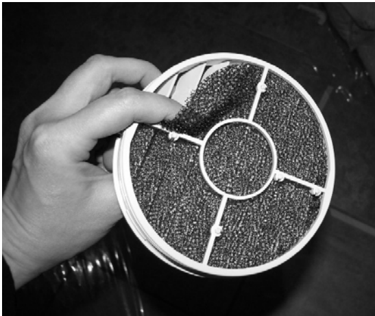
Air Filter (Located on back side of Return Air Vent)
