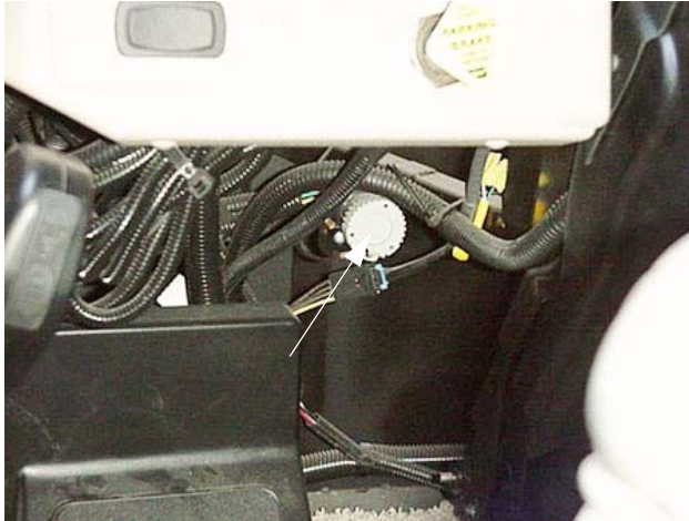
Diagnostic plug on steering column support beneath left side of dash -Typical View
