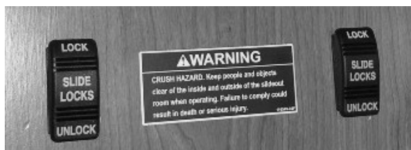
Slideout Room Travel Locks (Your model may be equipped with one or more types) -Typical View
