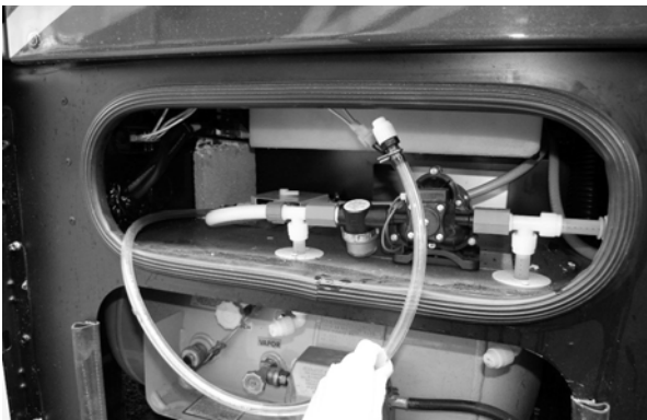
RV Antifreeze Siphon Tube (Located near water pump - second compartment on driver side of coach)
