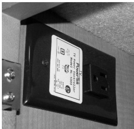
Front TV Ignition Switch Interlock -Typical View
