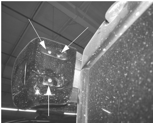
Entry Door Awning End Cap (Located on front inward end of Entry Door Awning)
