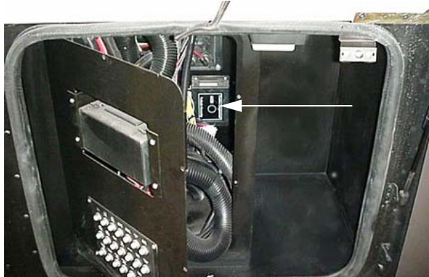
Keyless Entry Control Box (Located in 12-volt electrical compartment) -Typical View
