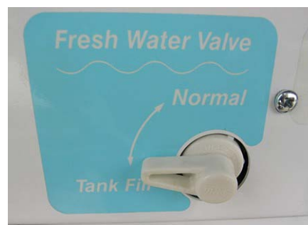
Fresh Water Valve in Tank Fill position (Located in water service center)
