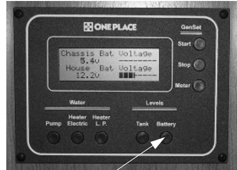
Battery Levels Switch
