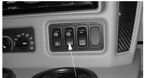
Coach Heat Switch -Typical View
