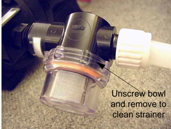
Water Pump Strainer -Typical View
