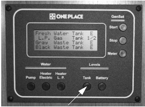
Tank Levels Switch
