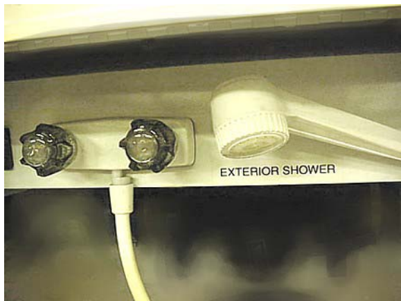
Exterior Shower/Wash Station -Typical View
