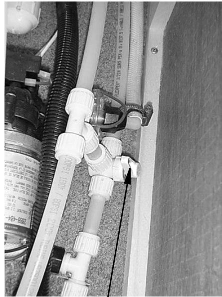
Waterline Drain Valve (Typical)
