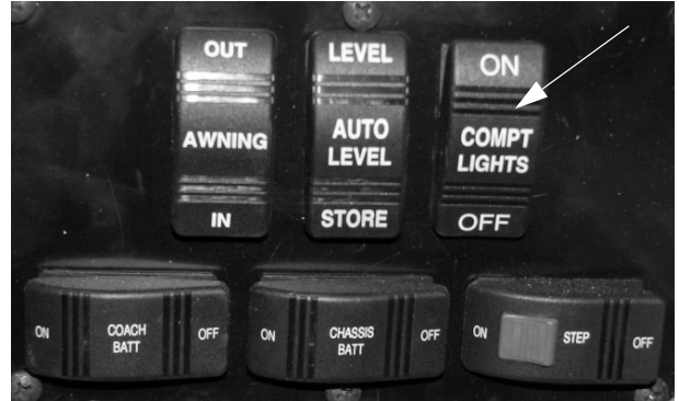
Compartment Lights Switch (Located near entrance door) -Typical View
