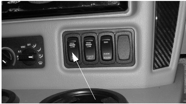
Defrost Fan Switch -Typical View
